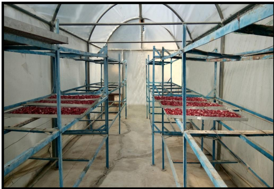
Plate 3. Drying of calyces of Roselle in solar tunnel dryer
