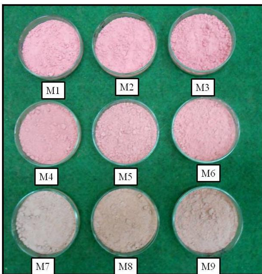
Plate 19. Microencapsulated Roselle anthocyanin powder obtained from different coating materials and inlet air temperatures
