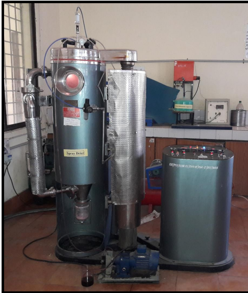
Plate 13. Spray dryer used for encapsulation of anthocyanin from calyces of Roselle
