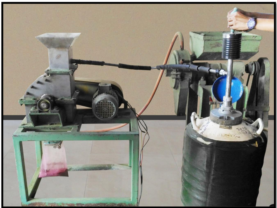
Plate 8. Liquid nitrogen (LN 2 ) cooled pulverizer
