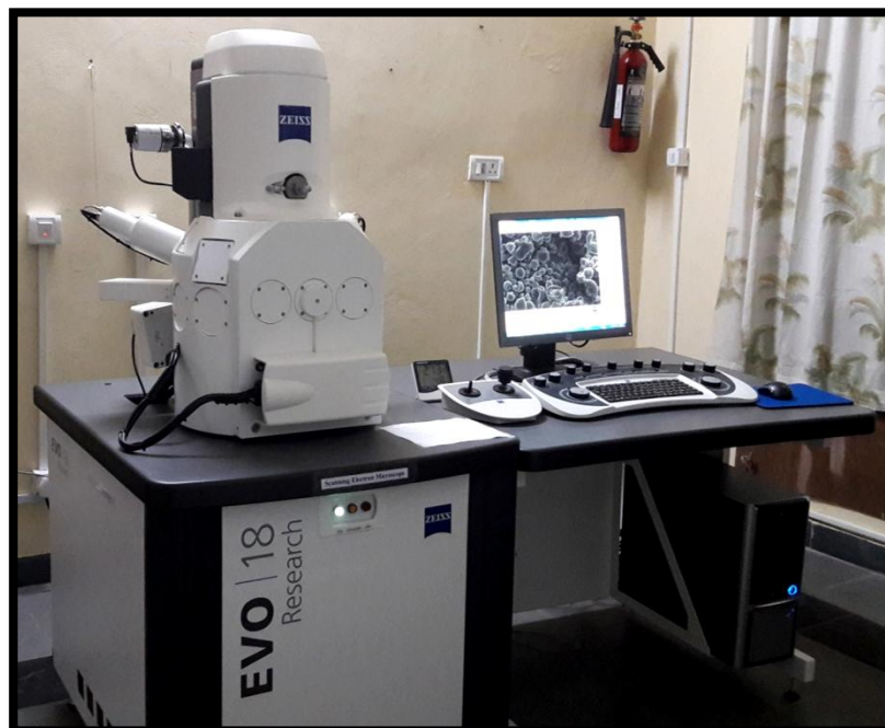
Plate 15. Scanning electron microscope for morphology of microencapsulated Roselle anthocyanin powder
