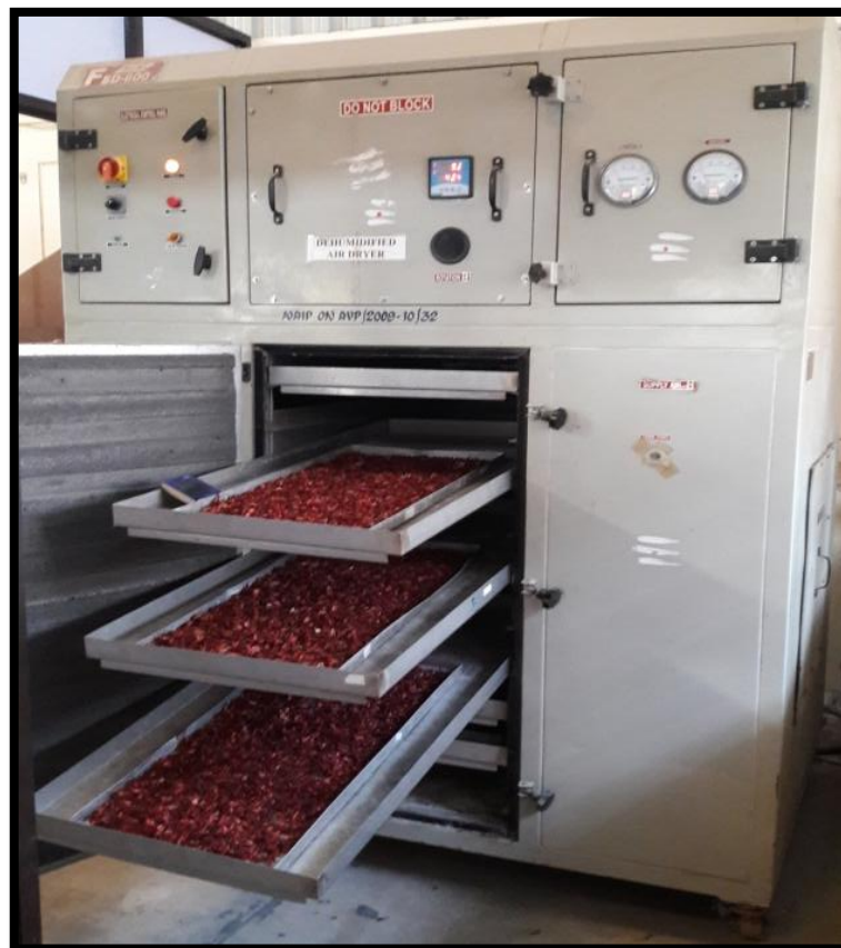
Plate 5. Drying of calyces of Roselle in dehumidified air dryer
