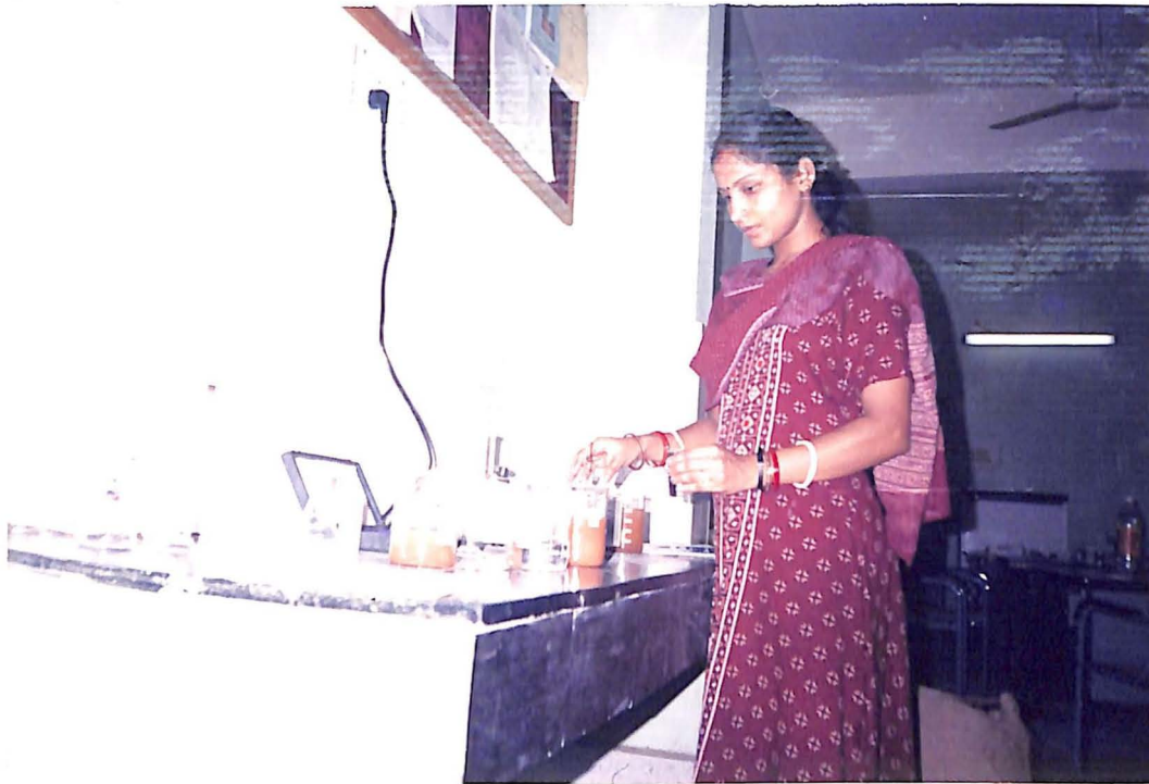
PLATE NO. 14. Measurement of filtration efficiency using Digital turbidity meter.
