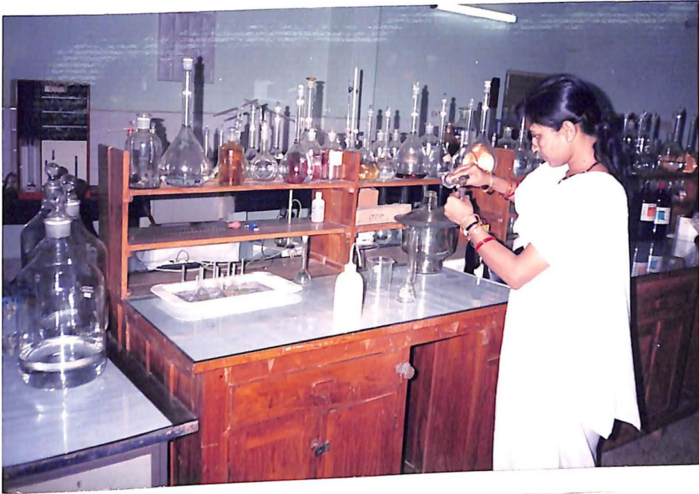
PLATE NO. 3. Preparation of standard turbidity suspension for calibration.
