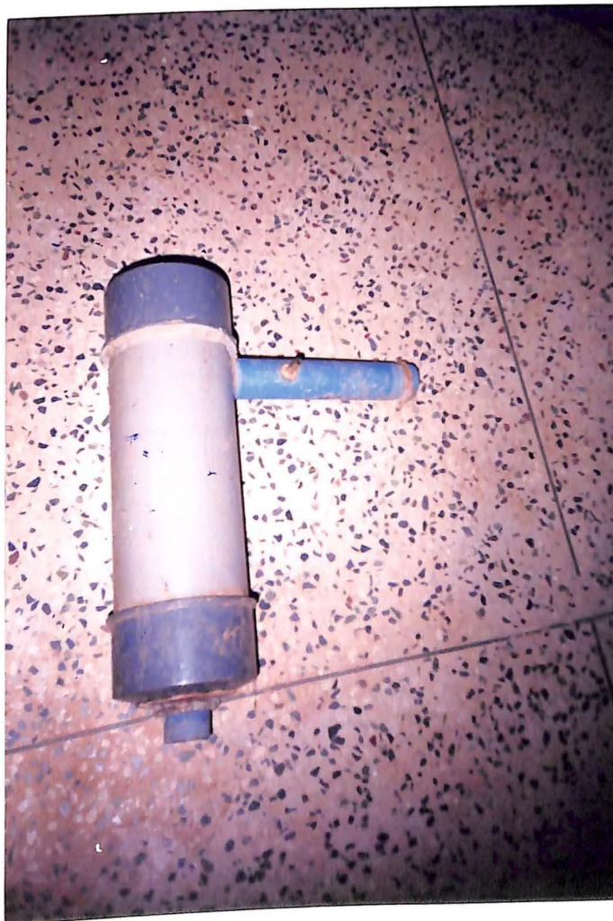
PLATE NO. 2. Low cost filter.
