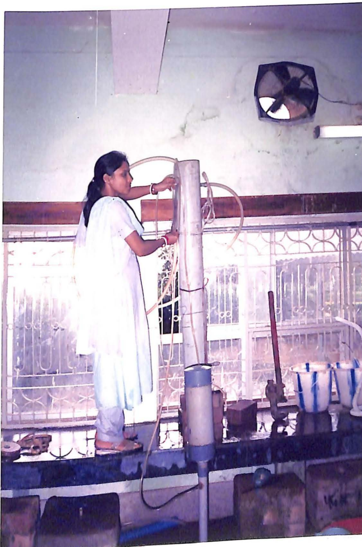
PLATE NO. 13. Measurement of head loss using water manometers.
