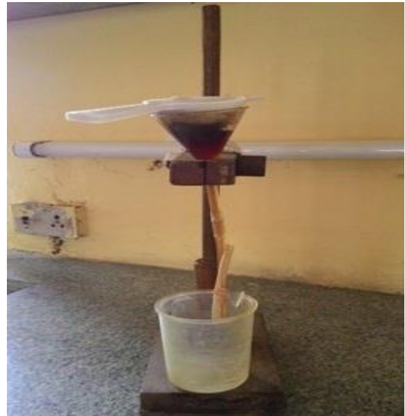
Plate 4.25b. Baermann's apparatus, for recovery of larvae
