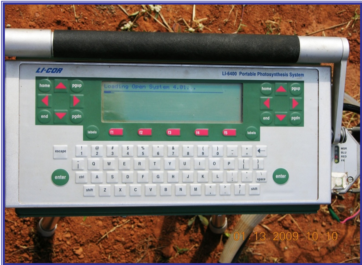
Plate 3.7: Infrared Gas Analyzer
