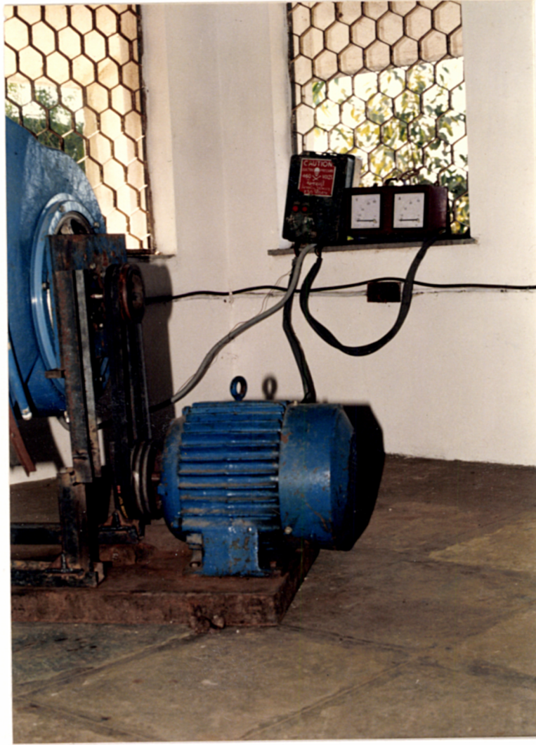
FIG. 4.10 SCHEMATIC VIEW OF BELT AND PULLEY ARRANGEMENT
