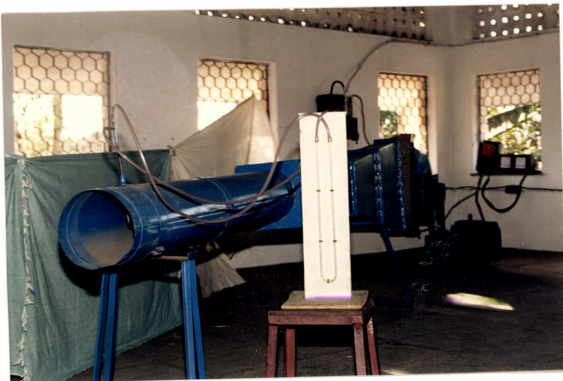
FIG. 4.11 SCHEMATIC VIEW OF PITOT TUBE CONNECTED WITH MANOMETER
