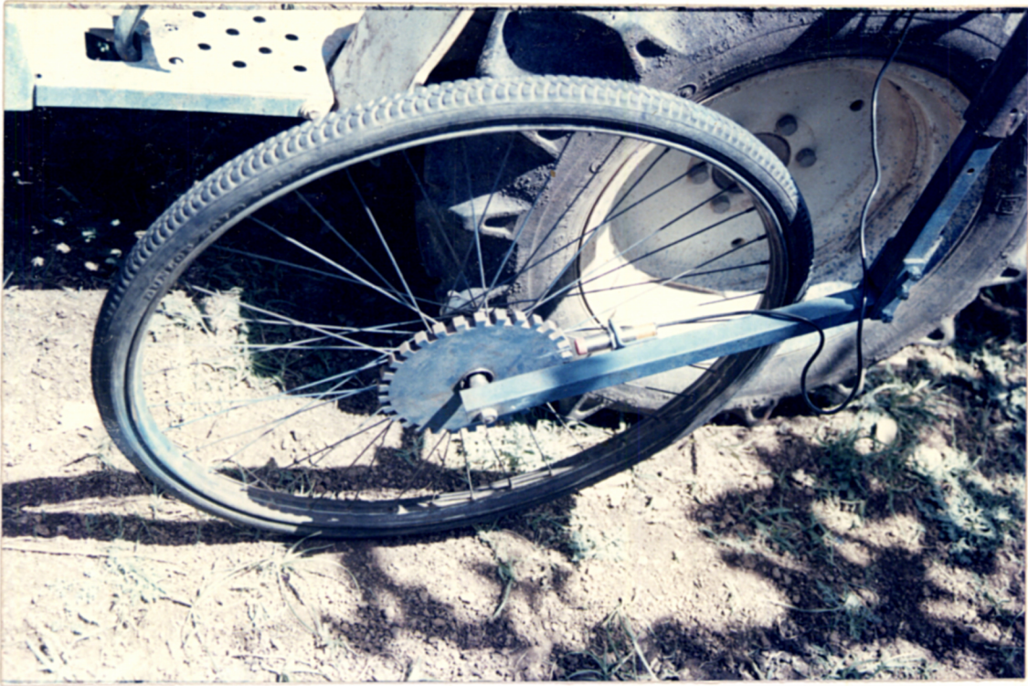
FIG. 4.24 BICYCLE WHEEL ATTACHMENT TO THE TRACTOR
