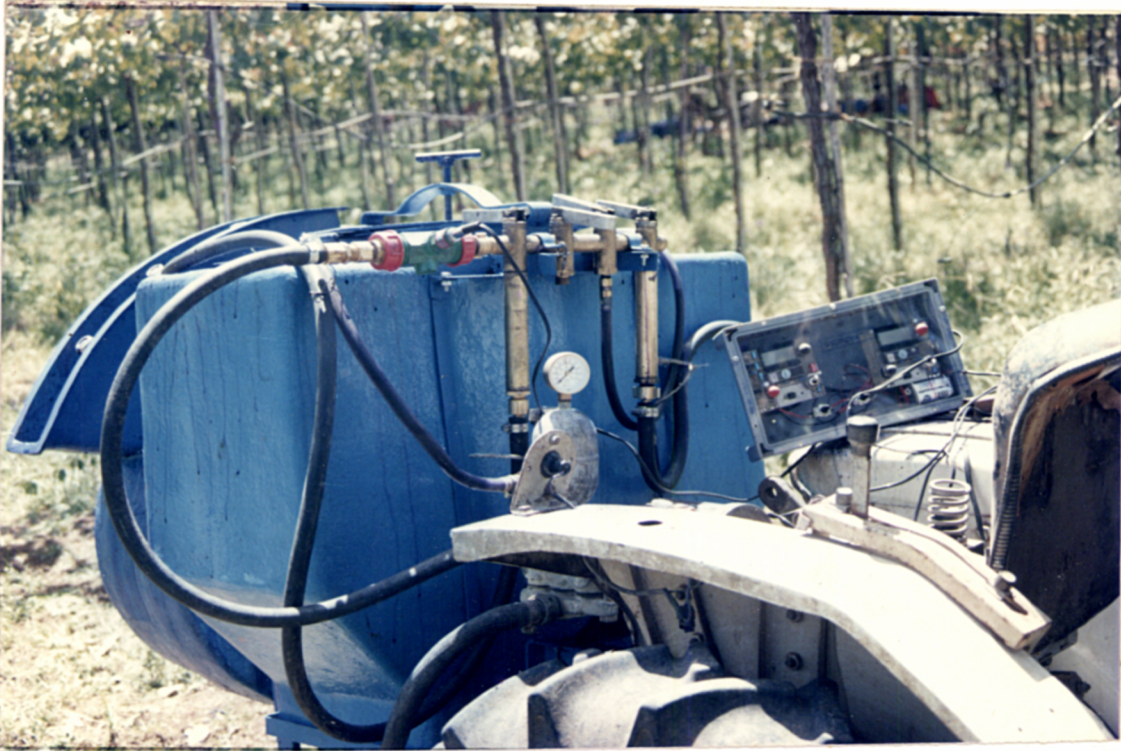
FIG. 4.18 CONTROL SYSTEM ON SPRAYER
