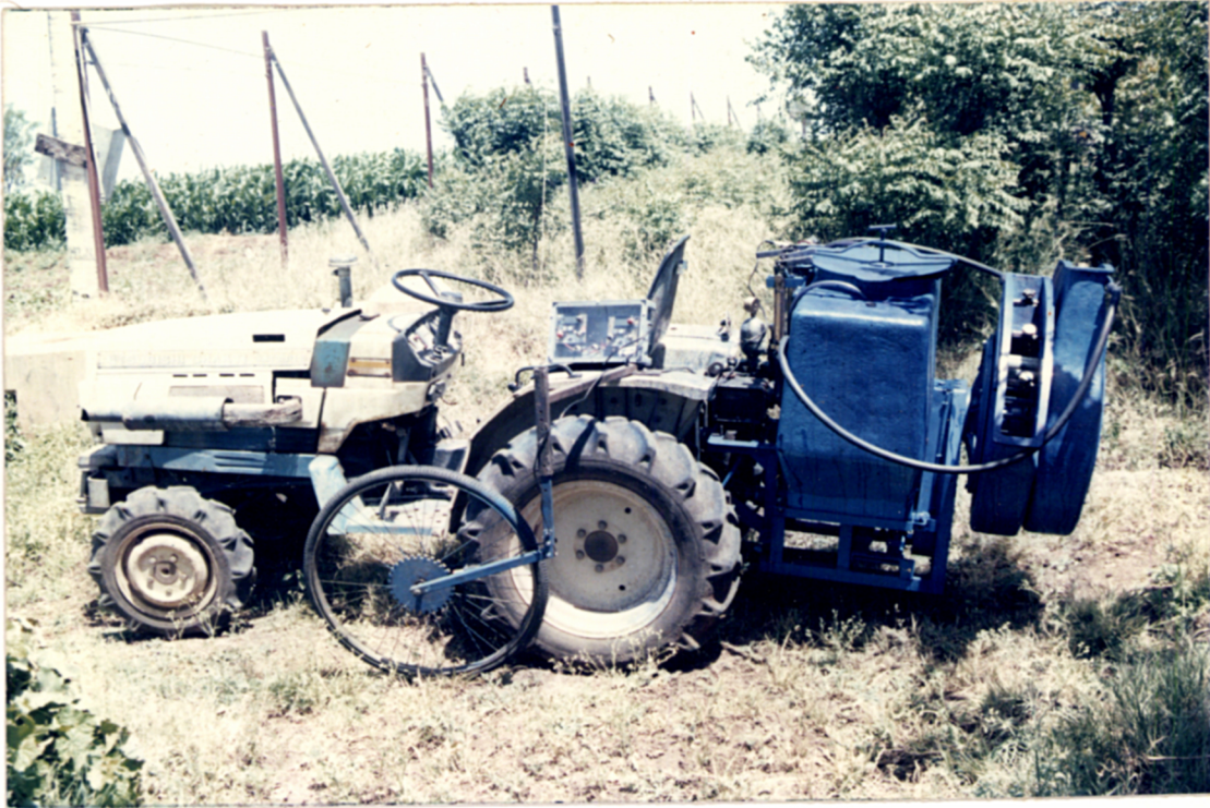
FIG. 4.1 TRACTOR MOUNTED AIR CARRIER SPRAYER
