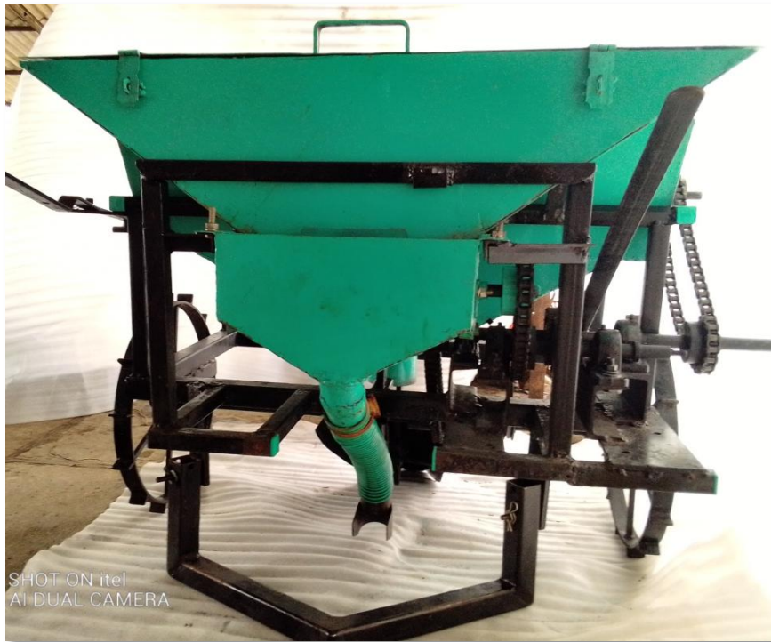
Fig. 3.23 Rear view of developed power weeder operated fertilizer application system for mango orchards
