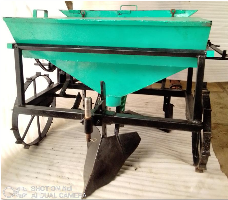
Fig. 3.21 Front view of developed power weeder operated fertilizer application system for mango orchards
