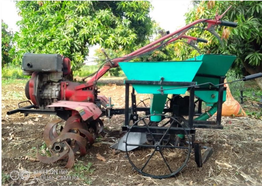
Fig. 3.25 Developed power weeder operated fertilizer application system for mango orchards
