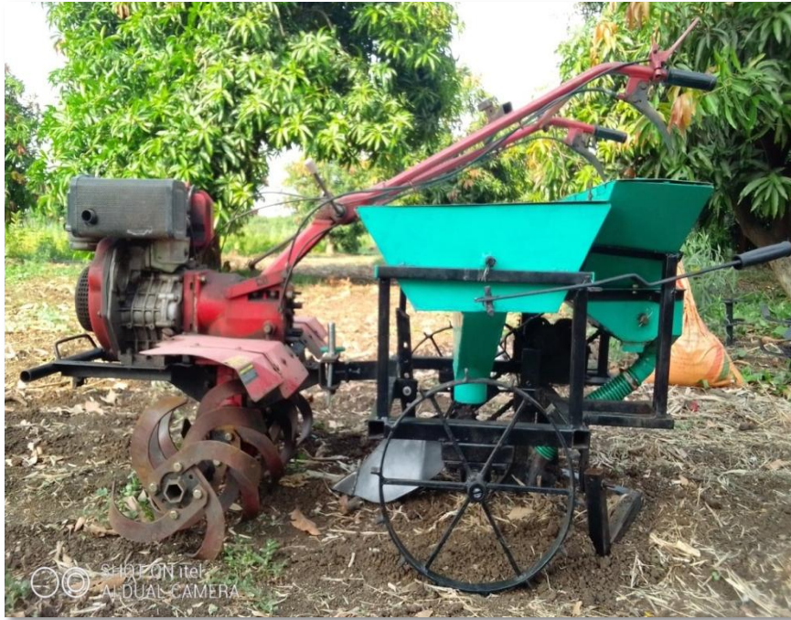
Fig. 4.1 Developed power weeder operated fertilizer application system for mango orchards
