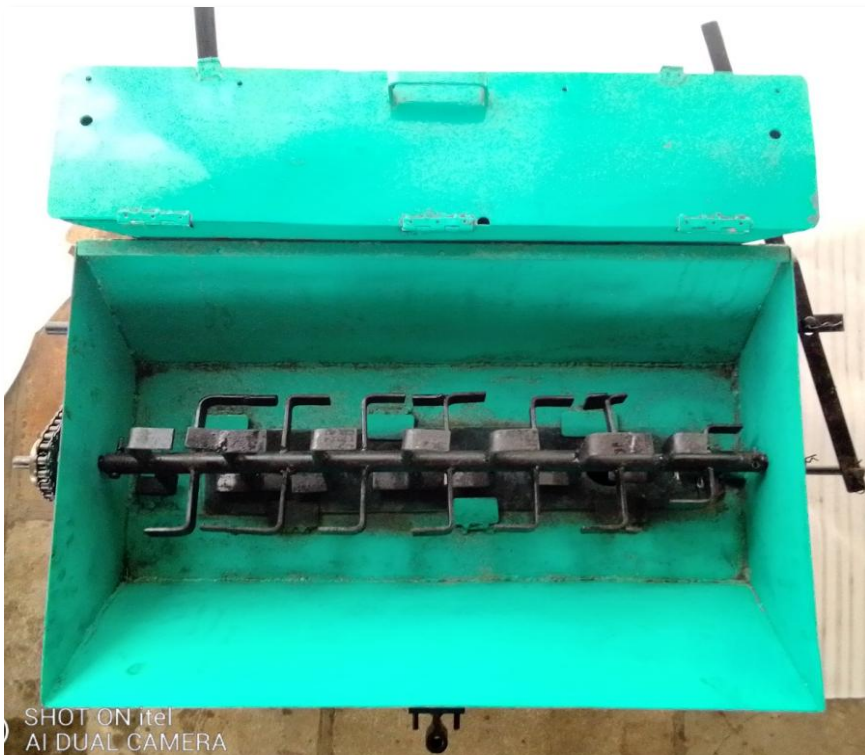
Fig. 3.22 Top view of developed power weeder operated fertilizer application system for mango orchards
