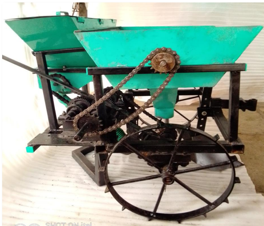
Fig. 3.24 Side view of developed power weeder operated fertilizer application system for mango orchards
