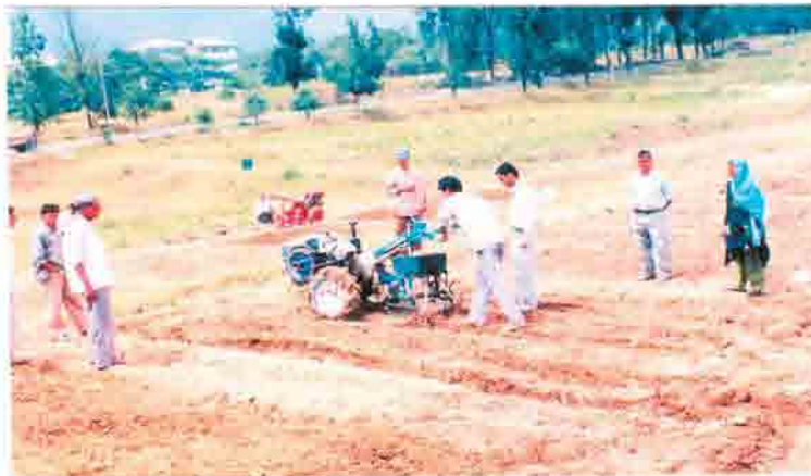
Sowing with power tiller operated zero tillage maize planter
