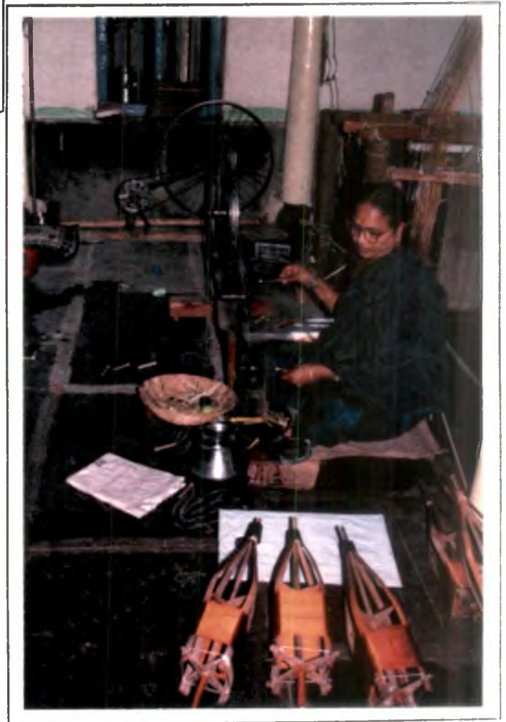
PLATE 11. PIRN WINDING OF SILK YARN
