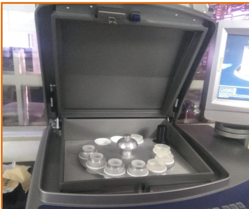
Plate 2: X-Ray Fluorescence machine for estimation of zinc and iron in rice grain
