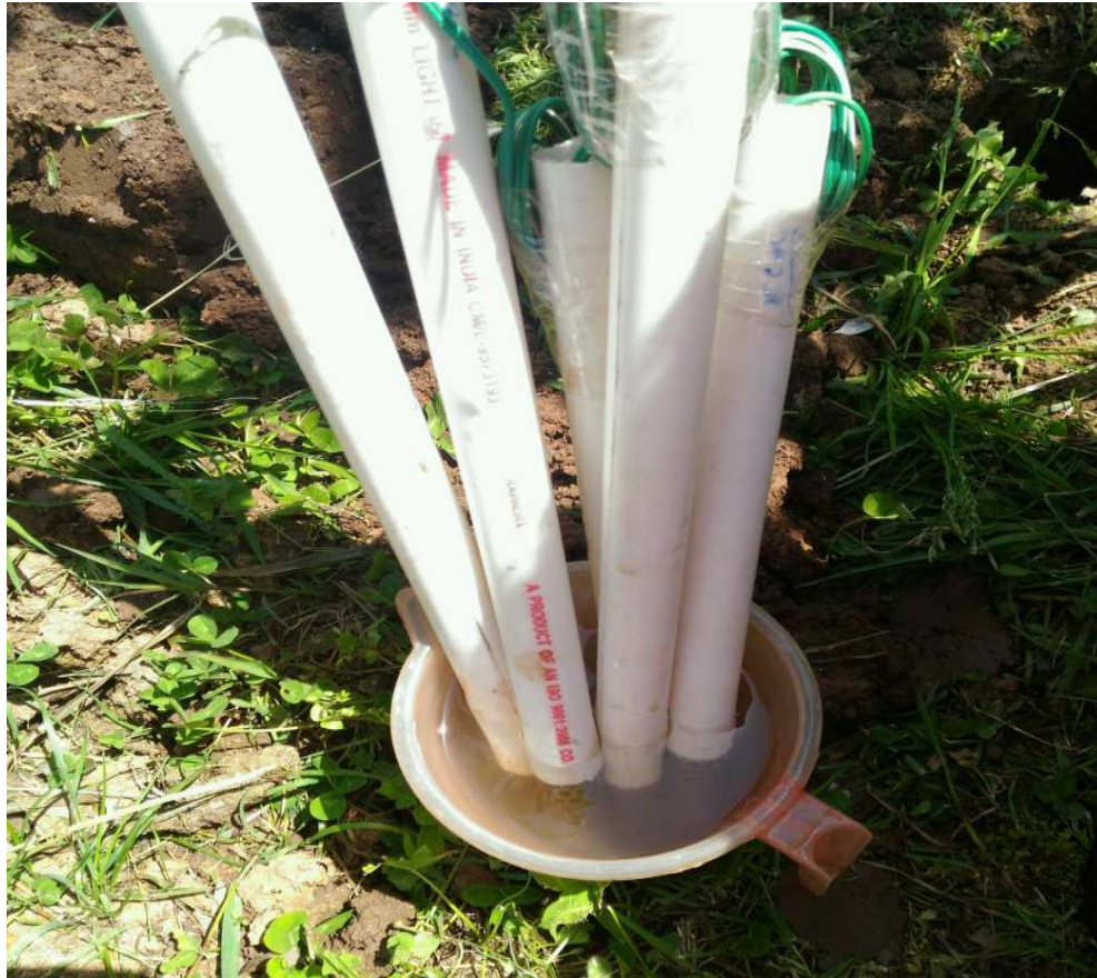
Plate 3.5: Sensors wetted before installing in soil
