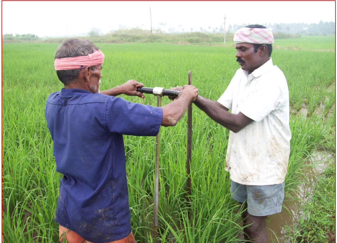
Plate 3.3 Inserting 2m deep auger for hydraulic conductivity measurement
