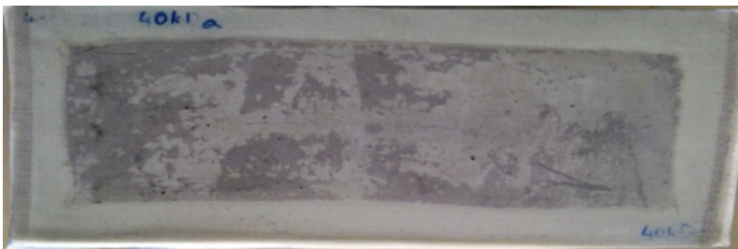
Plate 3.4 Ultrafiltration membrane of MWCO 40 kDa
