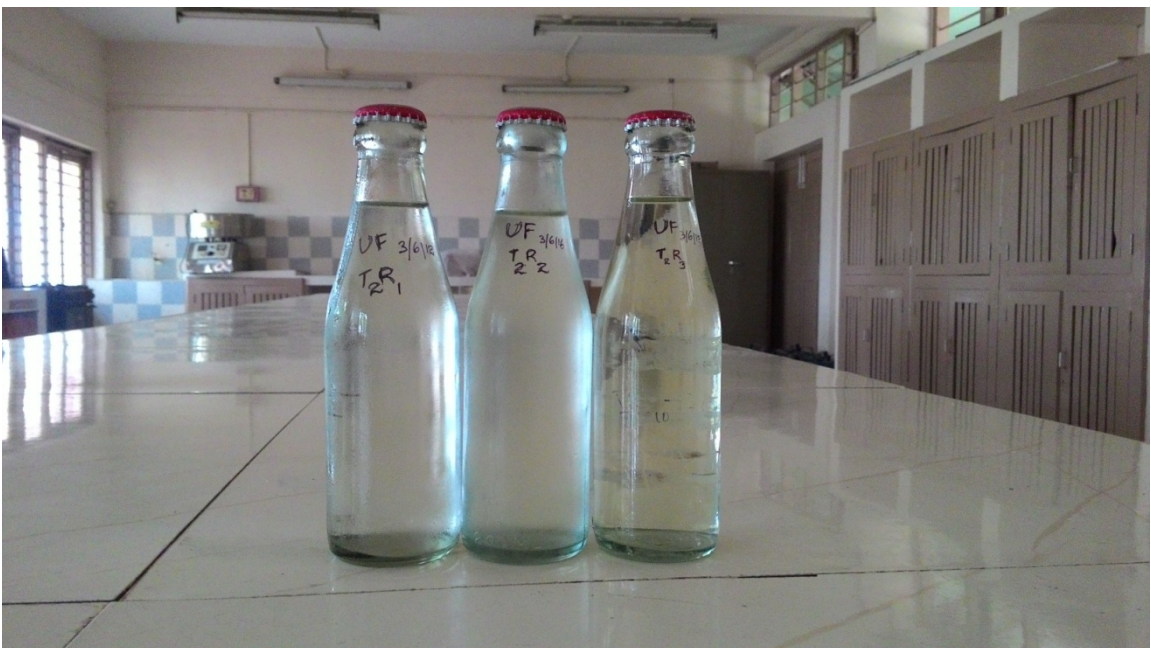
Plate 3.7 Ultrafiltered coconut water samples at a TMP 80 psi (5.06 kg/cm 2 )
