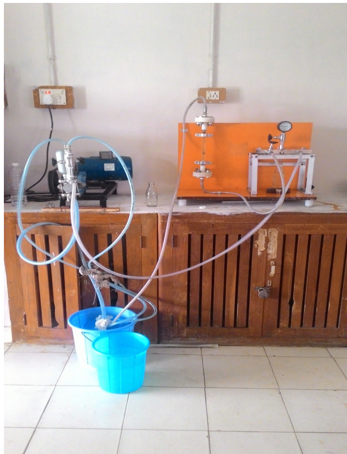
Plate 3.2 Cross flow cell membrane setup
