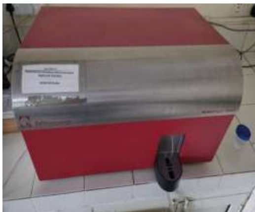
Fig. 10: Somatic cell counter used to measure SCC in milk samples
