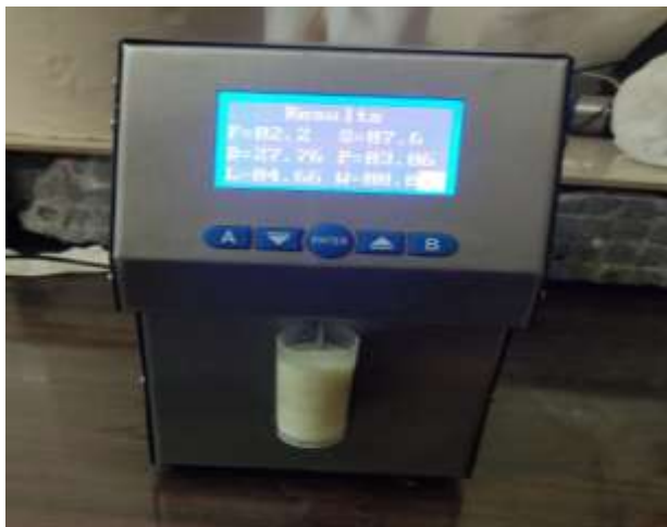
Fig. 9: Milk composition analysis by lactoscan milk analyser
