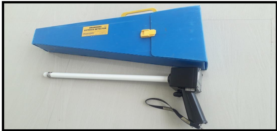
Plate 3.1 Device for Vaginal Electrical Resistance
