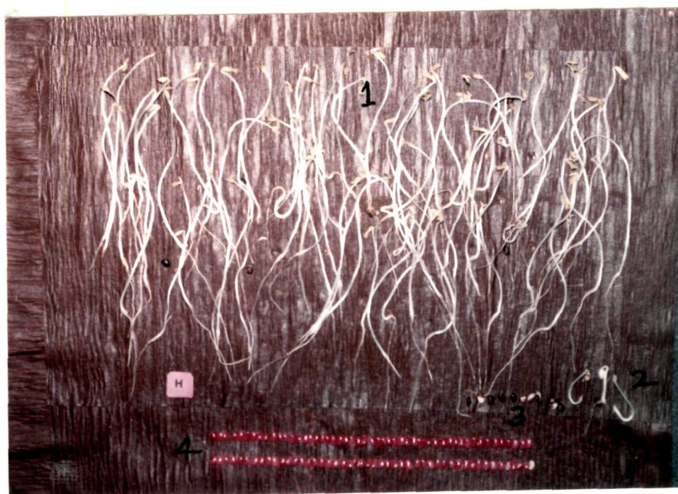
Plate 11: Standard germination and TZ test in horsegram
