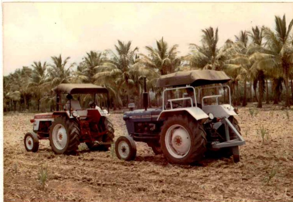
PLATE 3.12. MEASUREMENT OF FORCES ON IMPLEMENT THROUGH THREE DYNAMOMETER SYSTEM USING TWO TRACTORS
