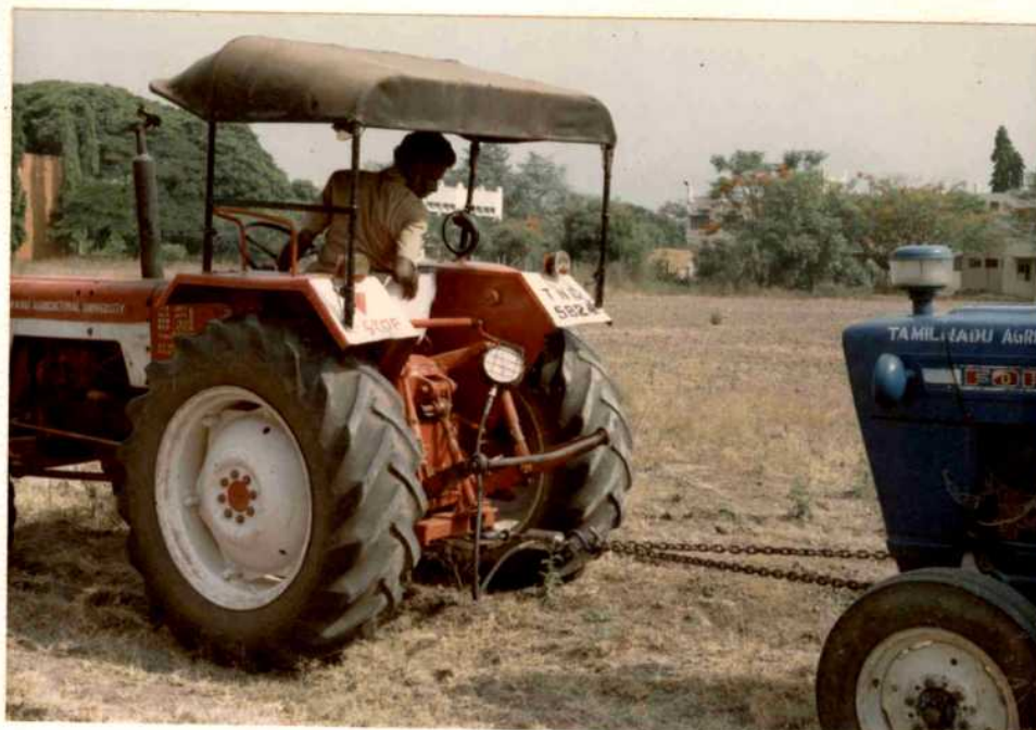
PLATE 3.13. HITCHING OF DYNAMOMETER BETWEEN TRACTORS TO MEASURE DRAFT
