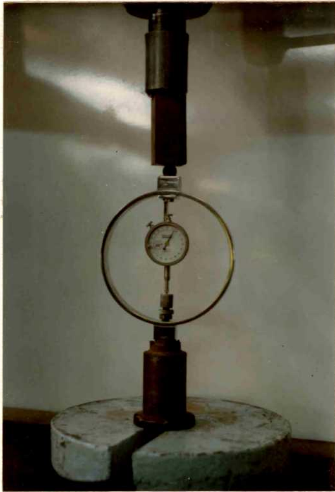
PLATE 3.5. CALIBRATION OF DYNAMOMETER USED IN TILLAGE DYNAMOMETER
