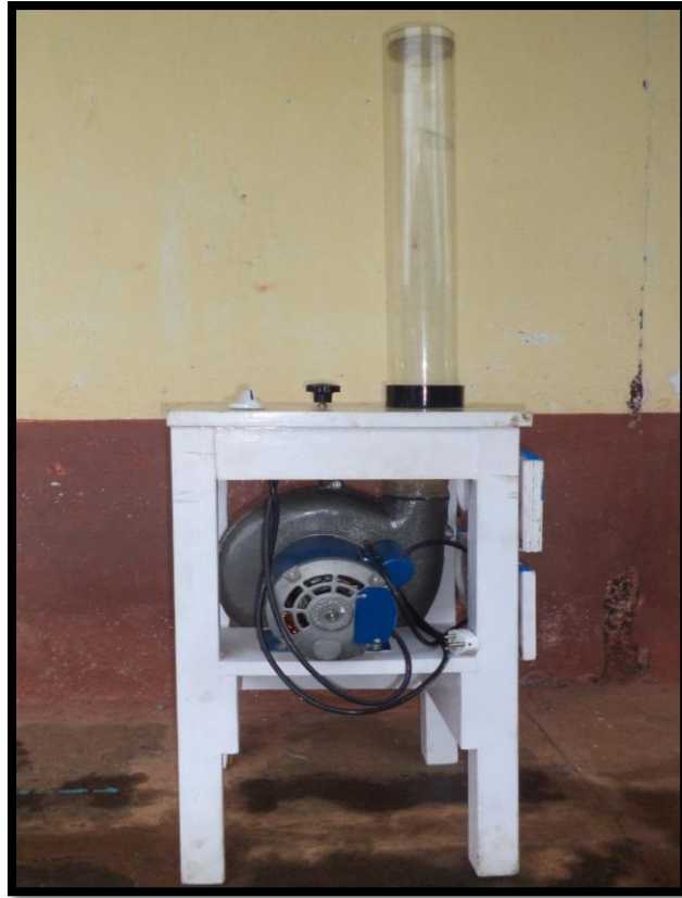
Plate 4.4 Seed Blower for Determination of Terminal Velocity
