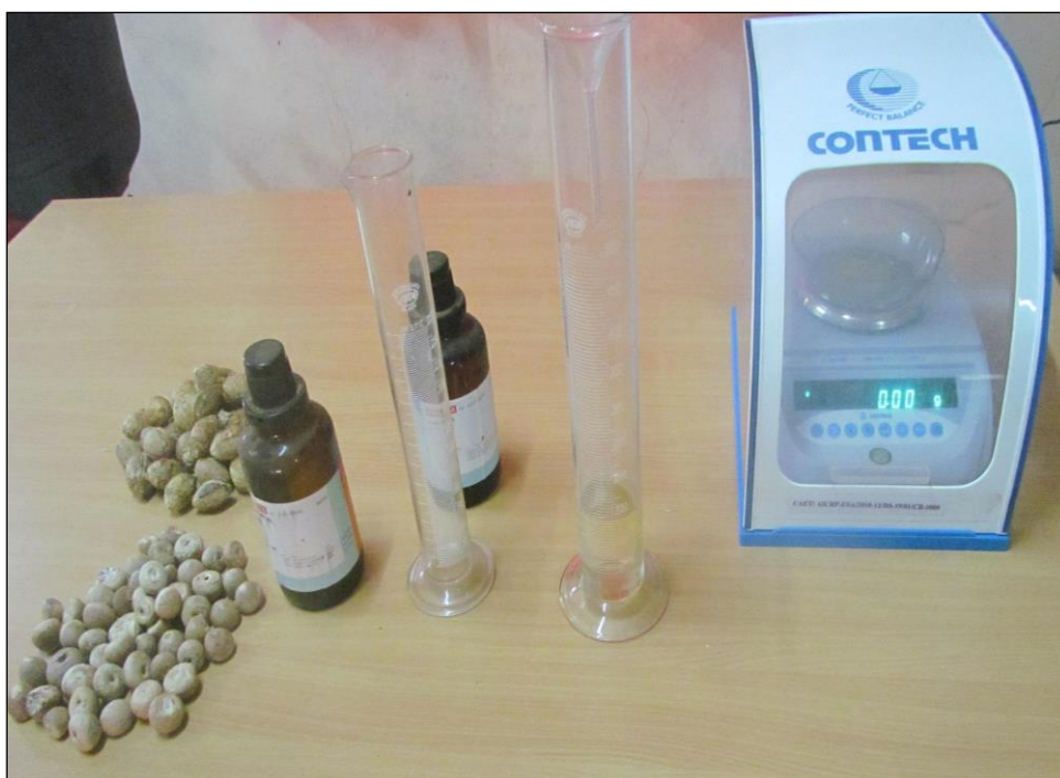
Plate 4.2 Set up for Determination of True Density of Arecanut Fruits and Kernel
