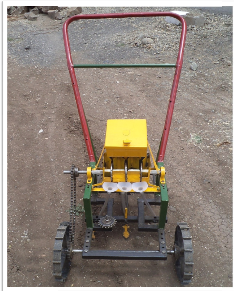
Plate 3.9 Manually operated onion seed planter
