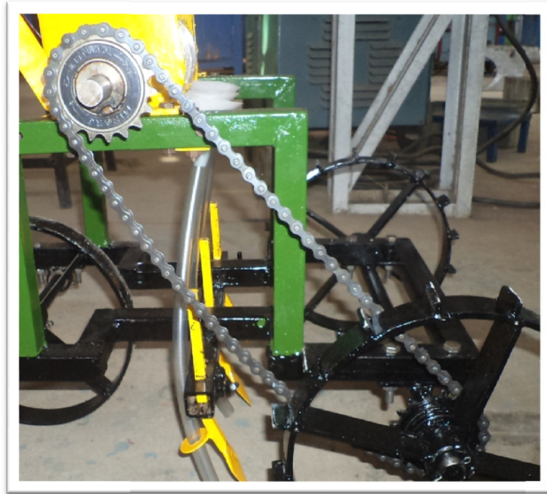
Plate 3.3 Chain and sprocket arrangement for power transmission from ground wheel to rotor shaft
