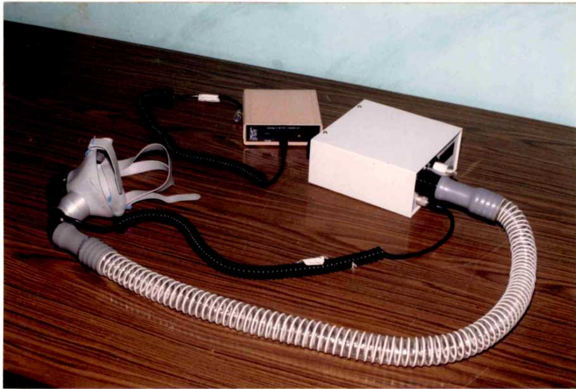
Plate 3.1 Oxylog-2 apparatus and its components
