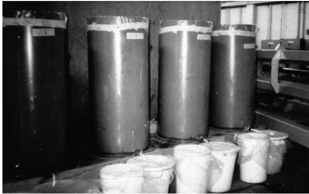
Figure 3 Column leaching facilities.
