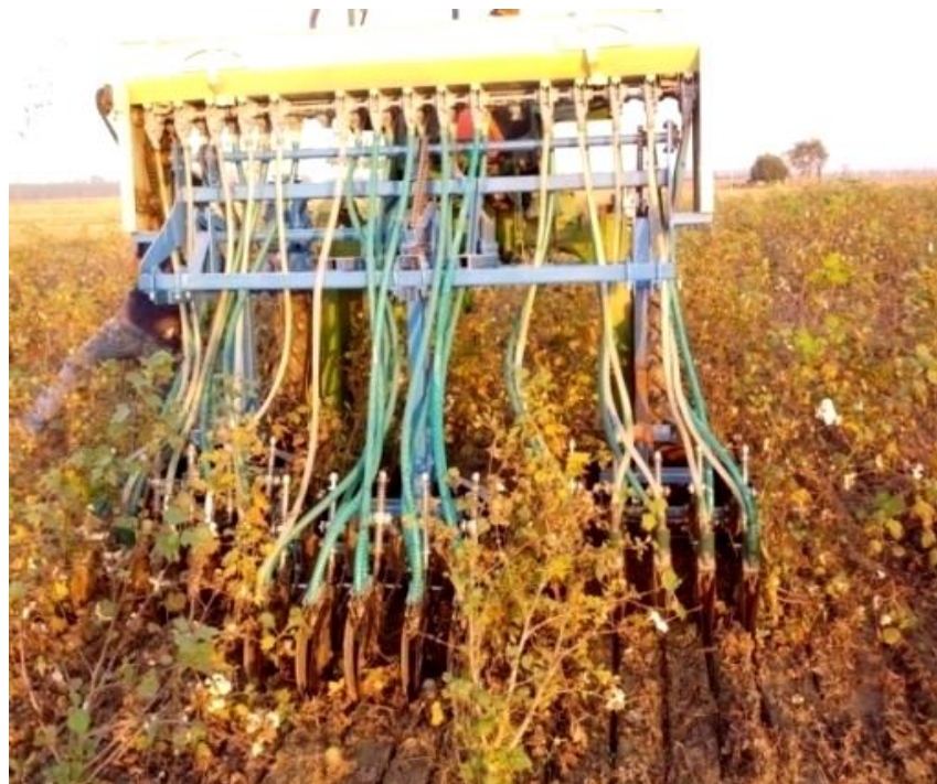
Fig. 4.5: 15-row relay seeder with ZTDD openers relay seeding wheat into standing cotton
