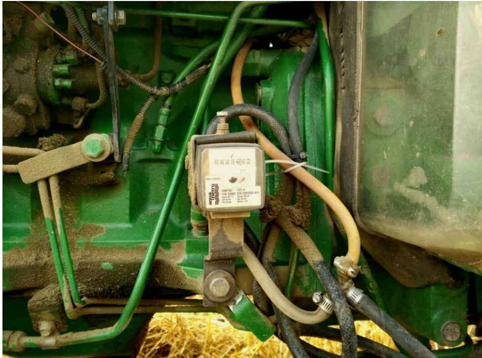
Fig. 3.23: Fuel flow meter installed in the fuel supply of tractor
