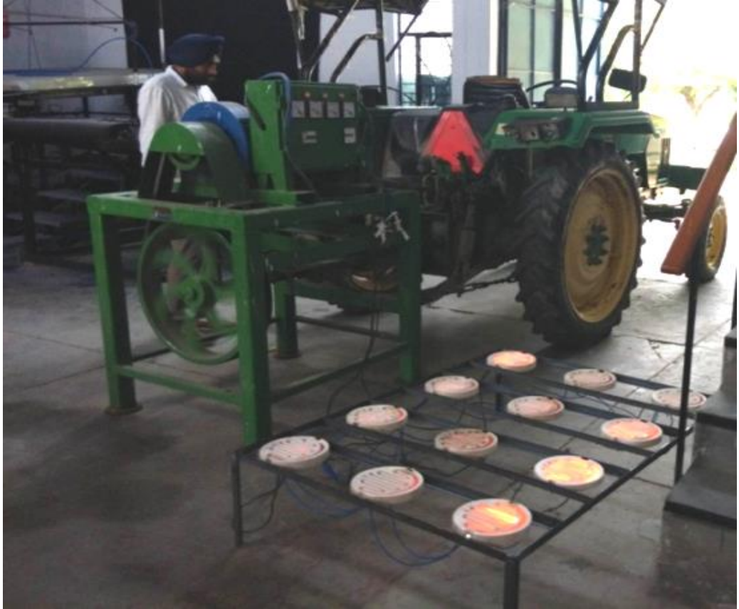
Fig. 3.24: Setup for measuring obtaining the power curve v/s fuel consumption
