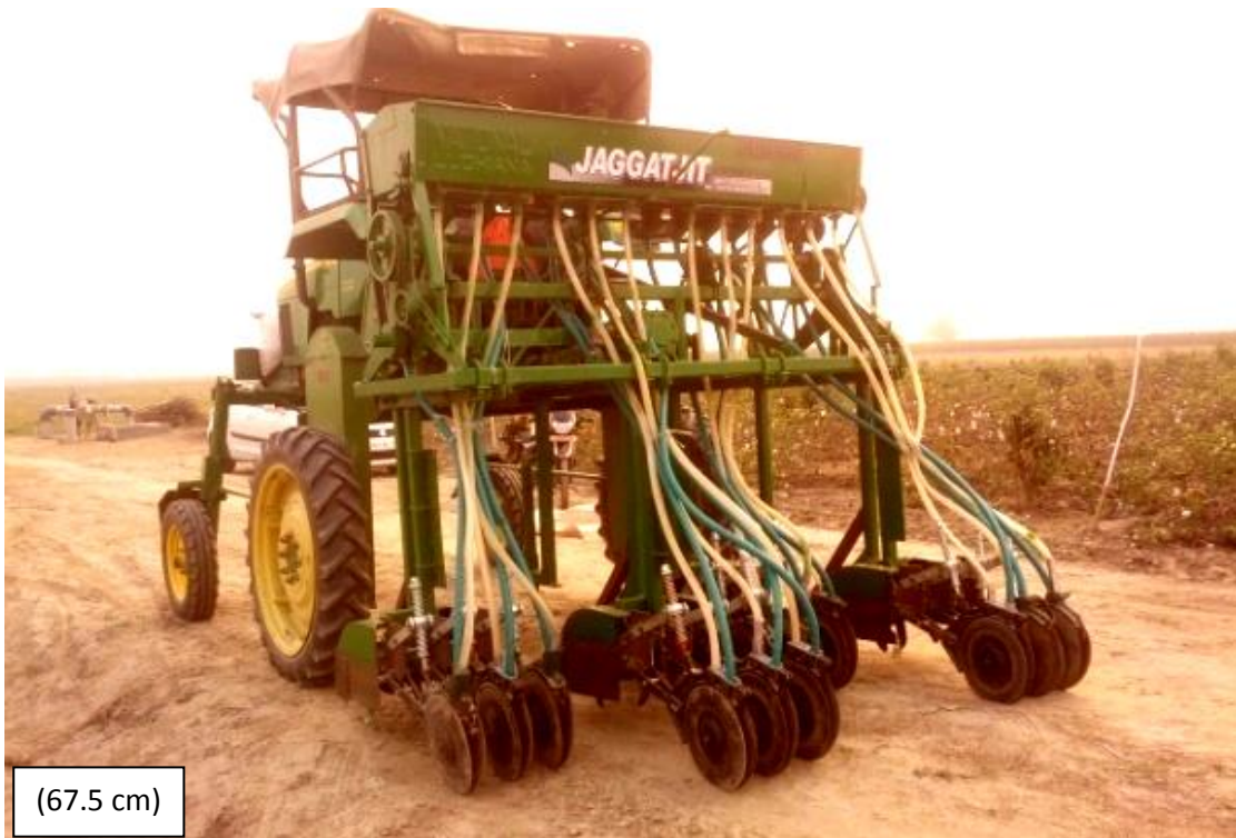
Fig 3.18: First prototype of 12 row relay seeder with ZTDD openers attached with the high clearance tractor
