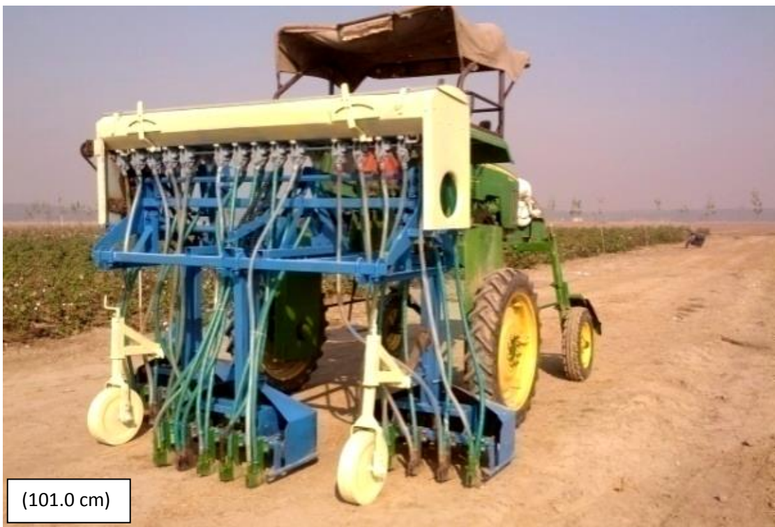
Fig 3.19: First prototype of 15 row relay seeder with ZTT openers attached with the high clearance tractor
