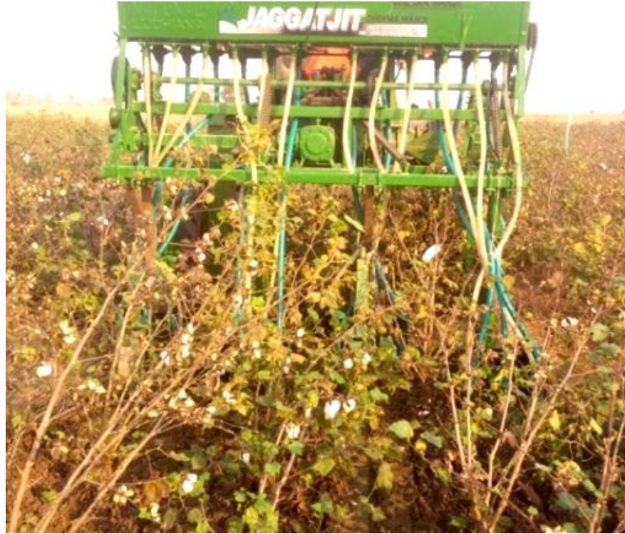
Fig. 4.4: 12-row relay seeder with ZTT openers relay seeding wheat into standing cotton
