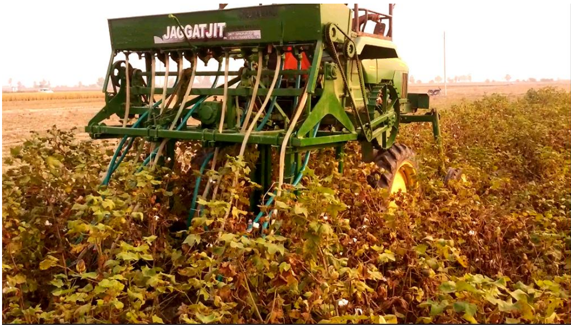
Fig. 4.18: 12-row Relay seeder with ZTDD furrow openers seeding wheat in cotton at Farmers field at Batinda, Punjab
