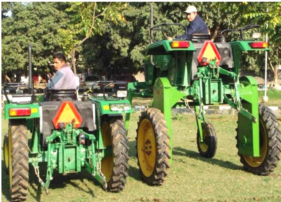
Fig. 3.2: Tractor (normal) and mounted on high clearance platform
