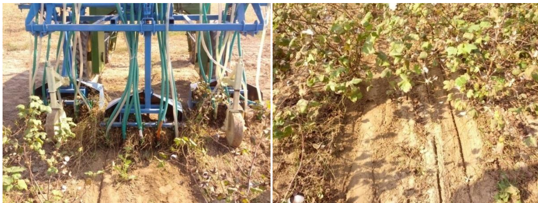
Fig. 4.9: Accumulation of weeds/plant residues on RS furrow openers and uneven sowing depth due to accumulation (from left to right)
