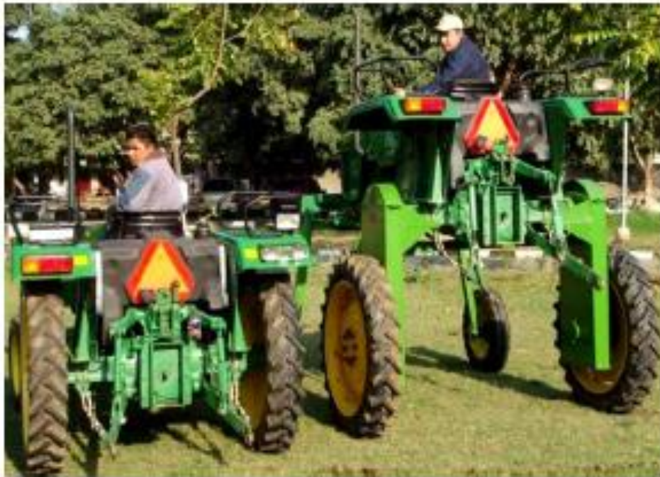
Fig. 1 Tractor (normal) and mounted on high clearance platform
