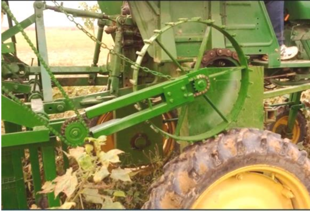
Fig. 3.16: Powering of driving wheel for seed and fertilizer metering mechanism from the rear tyre of tractor
