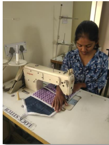
Finishing by piping
