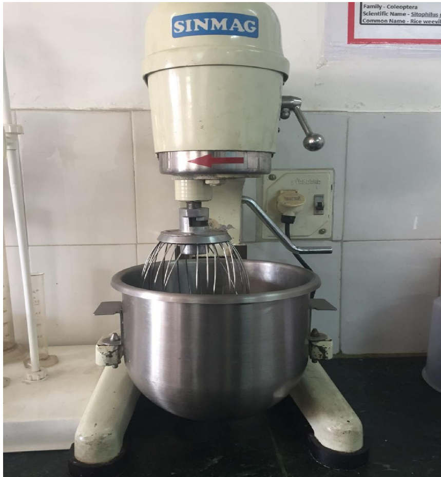
Plate 1: Planetary mixer used for flat bread preparation
