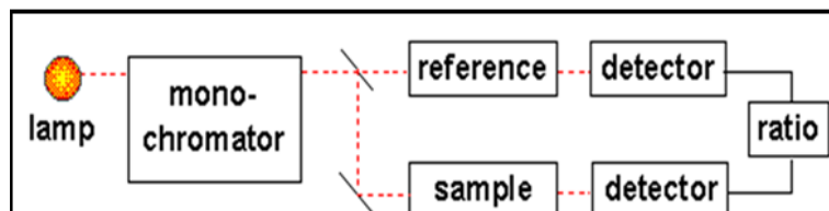
Figure 3.7: Schematic representation of UV-Vis Spectrophotometer
