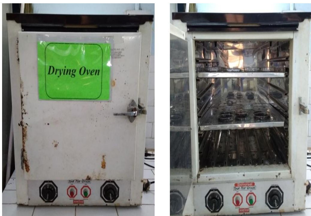
Fig.3.2: Moisture content determination by Hot air oven
