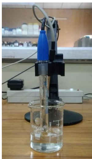
Fig. 3.8: Digital pH meter
