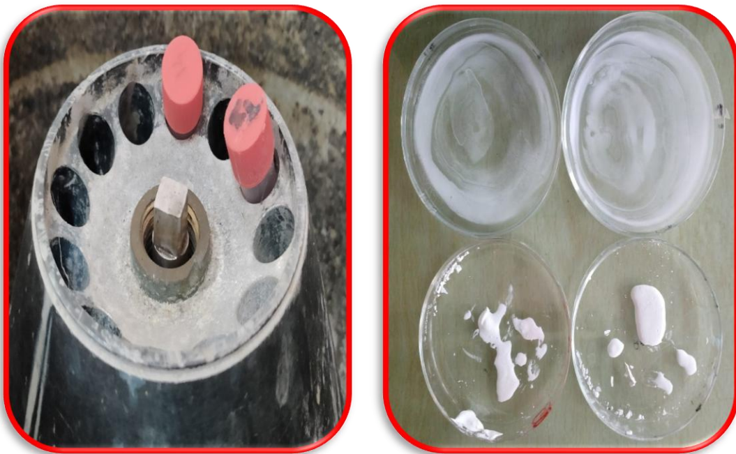
(B) Measurement of WAI and WSI
