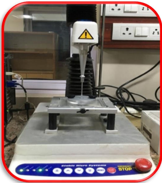
(B) Measurement of puncture strength of biodegradable film
