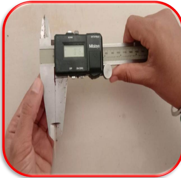
(A) Digital vernier caliper for measuring film thickness
