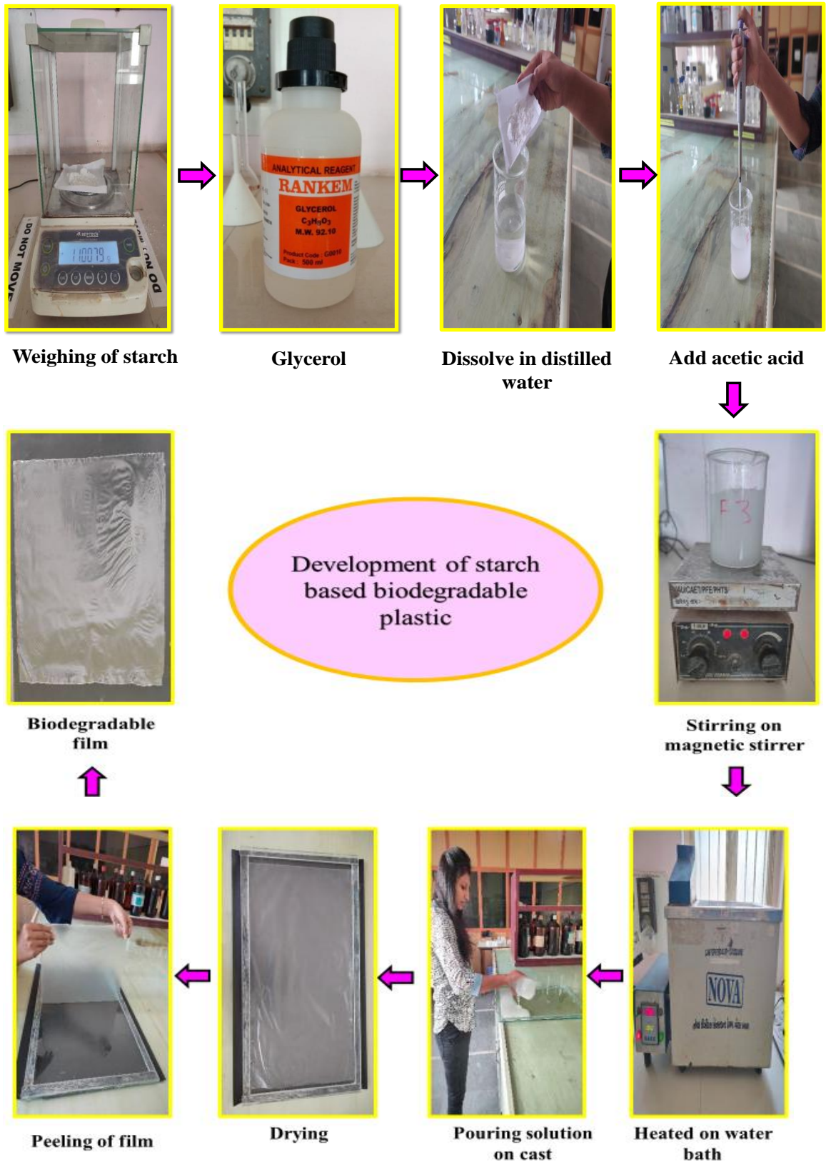
Plate 3.3: Pictorial process flow chart for development of biodegradable plastic
