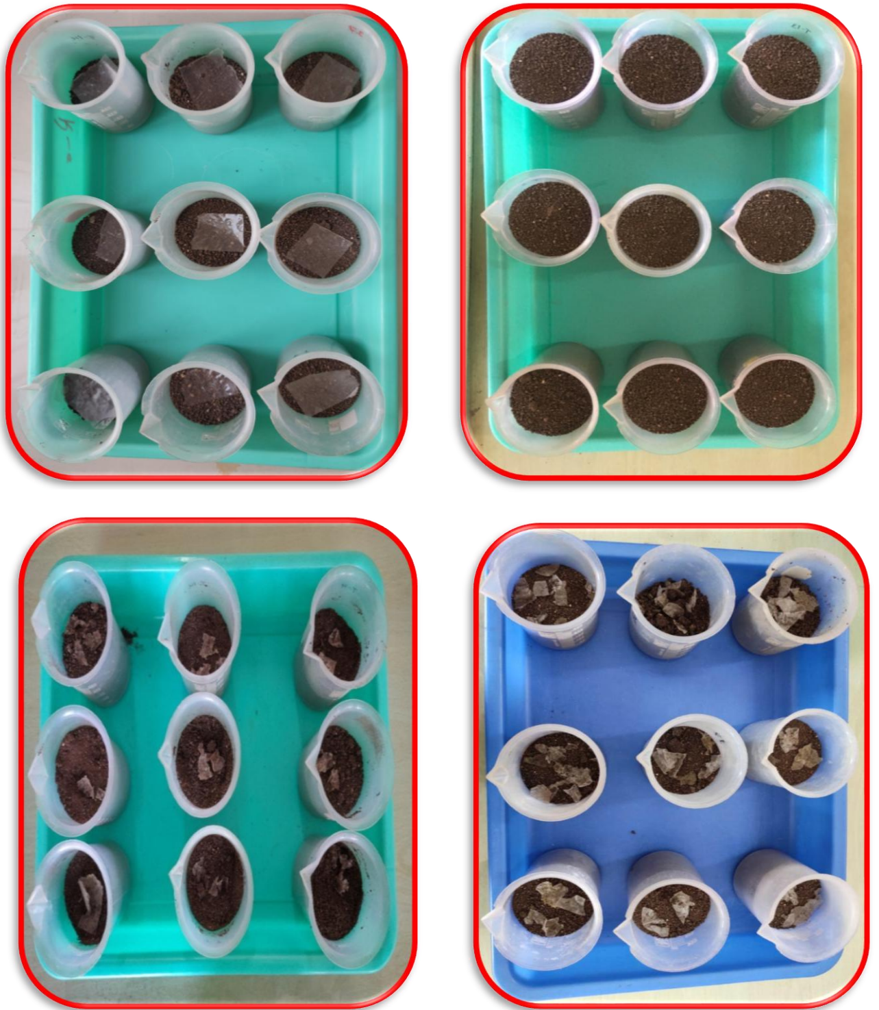
Plate 3.7: Measurement of biodegradation properties of biodegradable film
