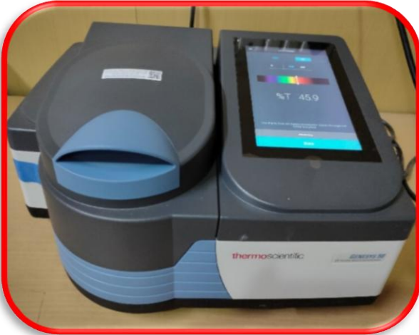
(B) Measurement of transparency by using spectrophotometer
