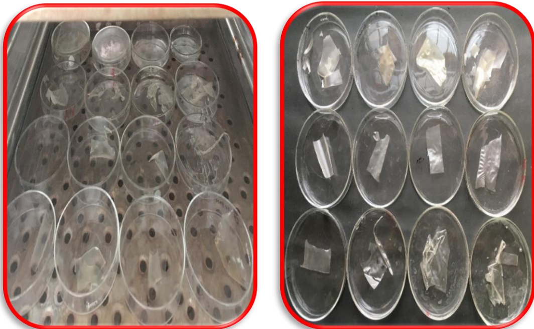
(B) Hot air oven used for determination of moisture content
