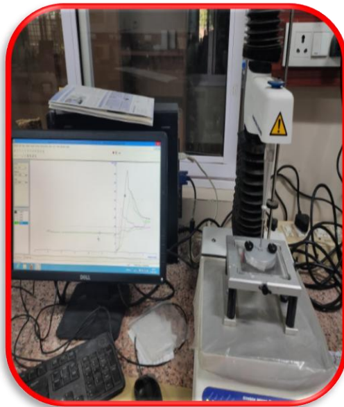
(B) Measurement of puncture strength of biodegradable film
