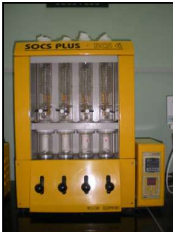
Fig. 3.2: Soxhlet apparatus for fat estimation
