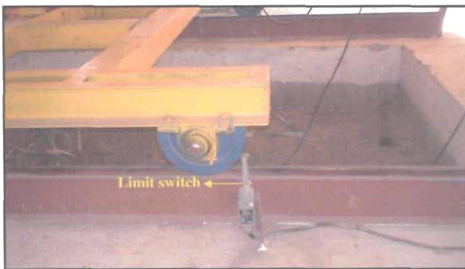
Fig. 3.6 Lever type limit switch
