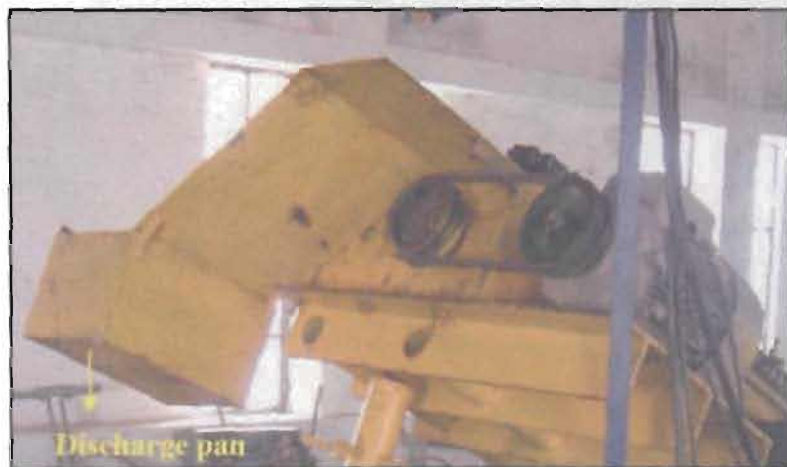
Fig. 3.17 Discharge pan to collect the picked cobs
