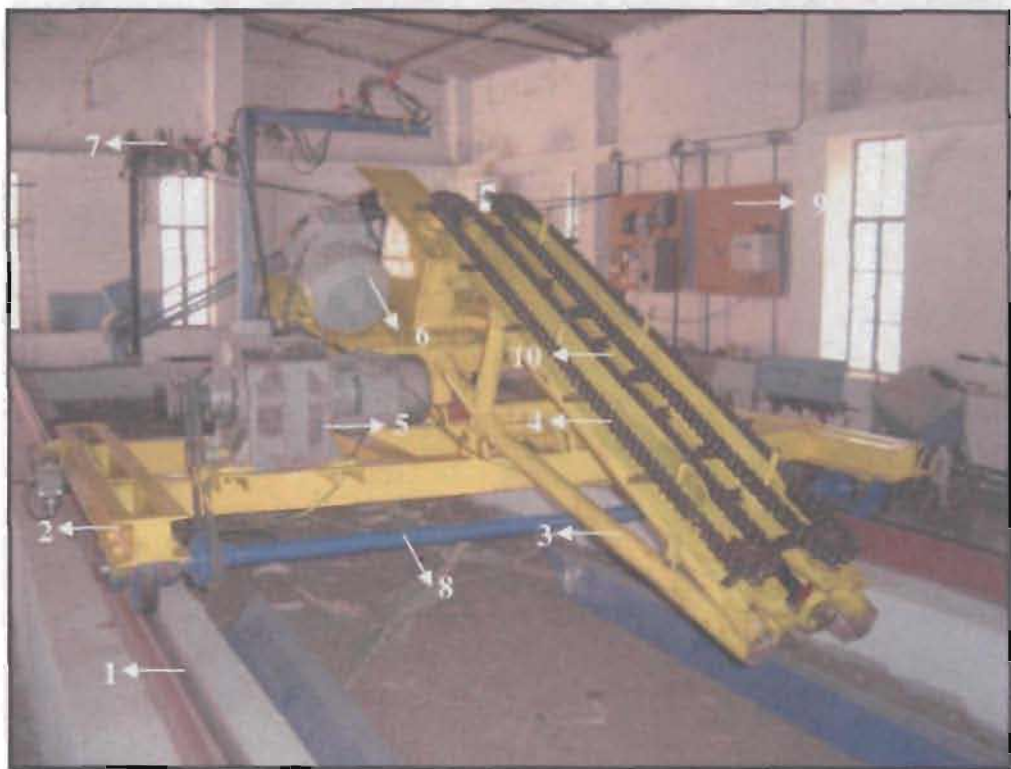
Fig. 3.21 A view of developed corn picking mechanism
