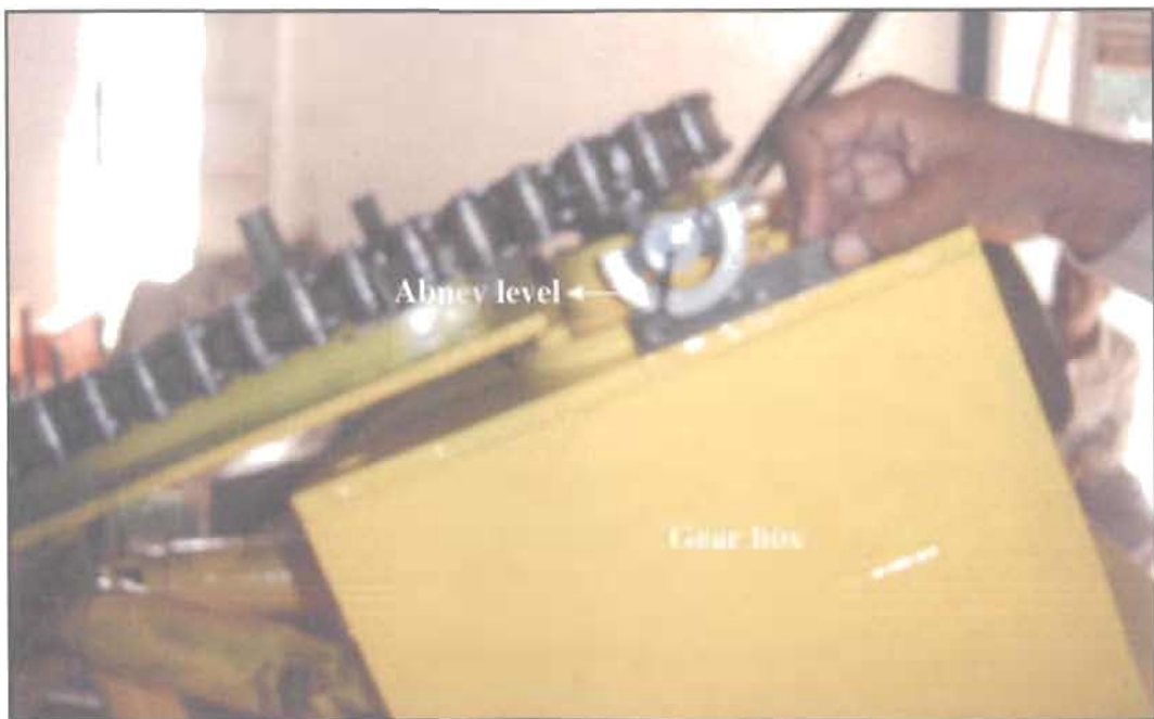
Fig. 3.23 Measurement of angle inclination with the help of Abney level
