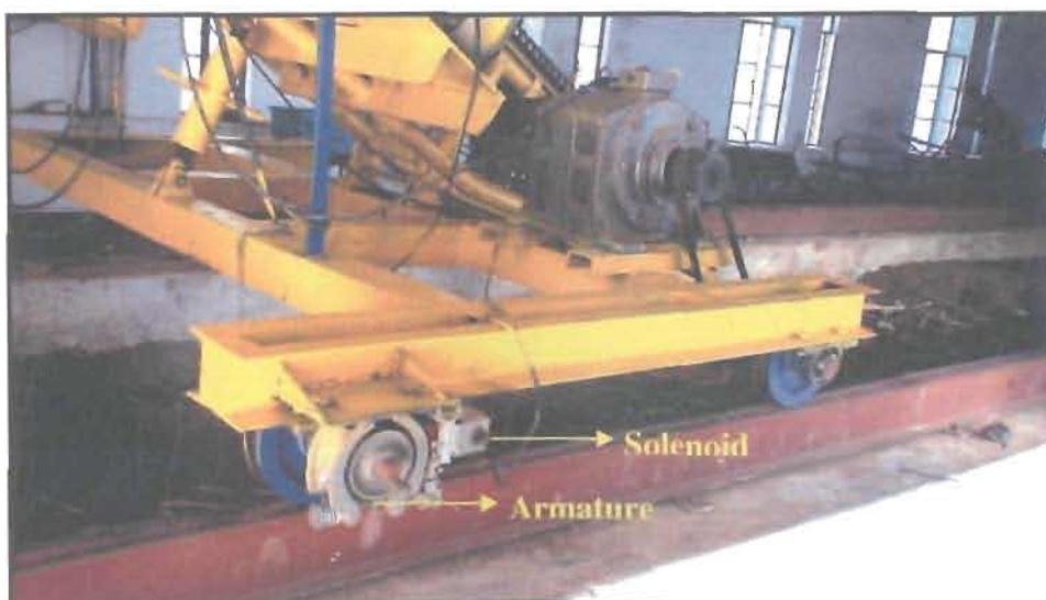
Fig 3.7 Brake system used in mounting trolley
