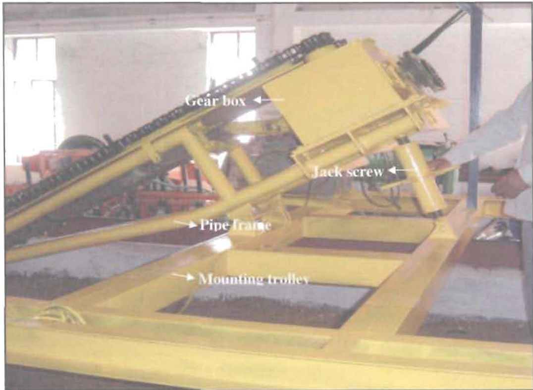
Fig. 3.22 Change of angle of inclination of snapping rolls with Jack screw
