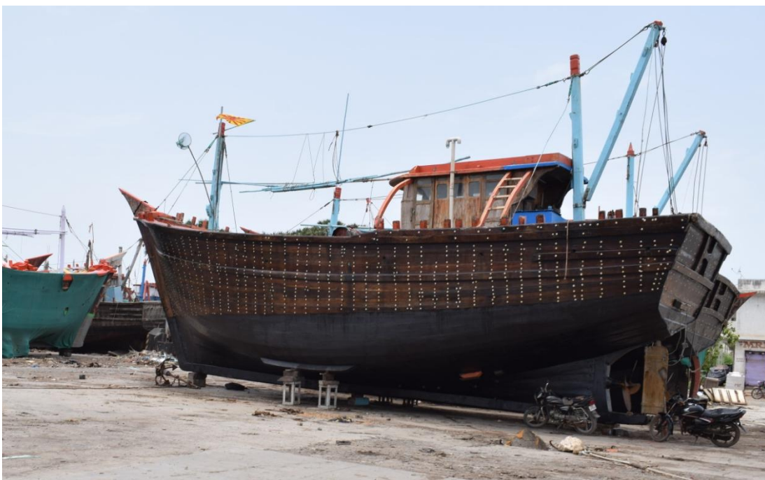
Plate 4.1.1.1 (b) Multi-day trawler under construction at Veraval, Gujarat
