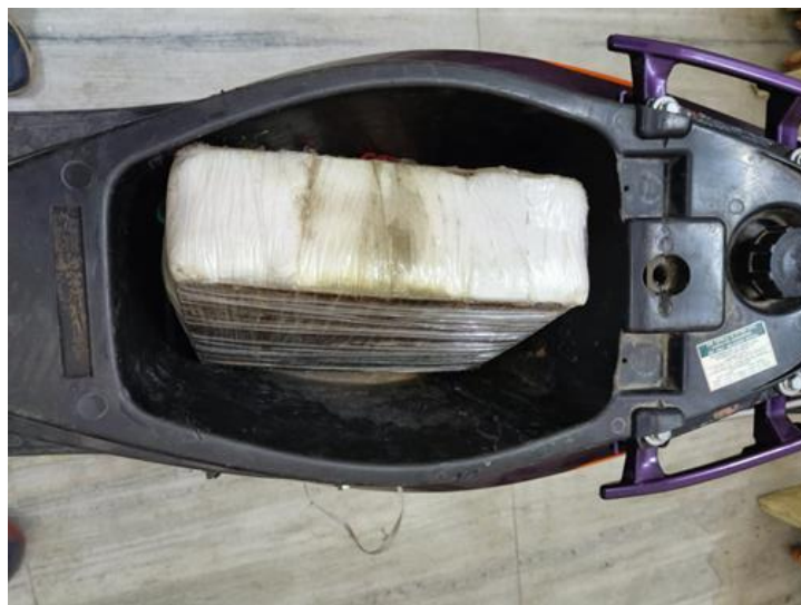
Fig 3.5 Battery pack placed in the boot of Hybrid Electric Scooter
