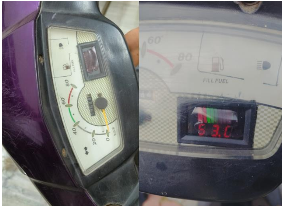
Fig 3.8 Voltage display placed on console of Hybrid Electric Scooter
