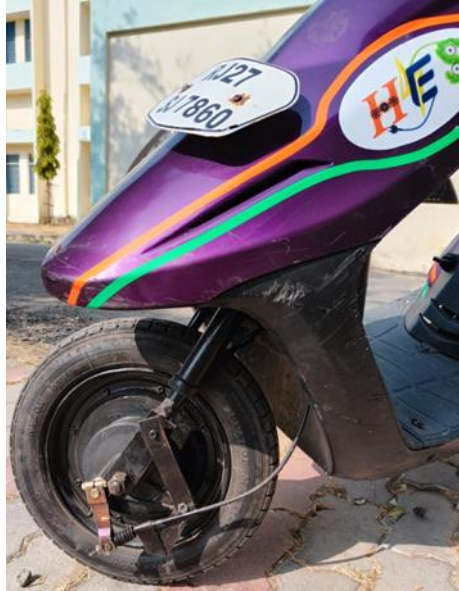
Fig 3.4 In wheel hub BLDC motor placed on Hybrid Electric Scooter
