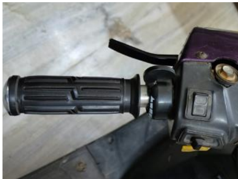
Fig 3.7 Throttle placed at the left hand grip side of Hybrid Electric Scooter
