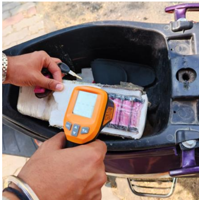
Fig 3.12 Using temperature gun to measure battery temperature
