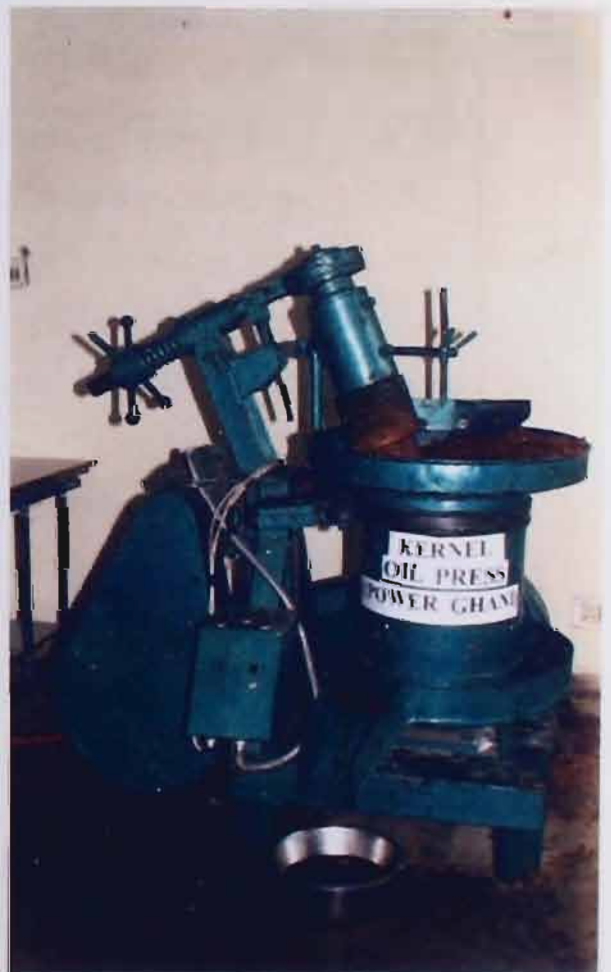
Plate 6. OIL PRESS: (a) CONTACT PARTS MADE OF SS (b) CONTACT PARTS MADE OF WOOD
