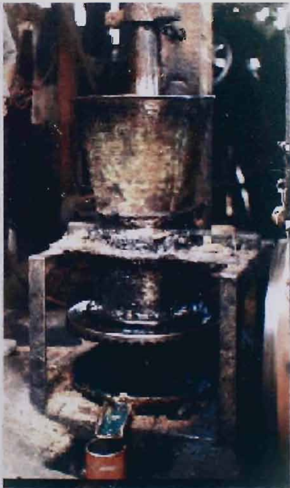
Plate 6. OIL PRESS: (a) CONTACT PARTS MADE OF SS (b) CONTACT PARTS MADE OF WOOD
