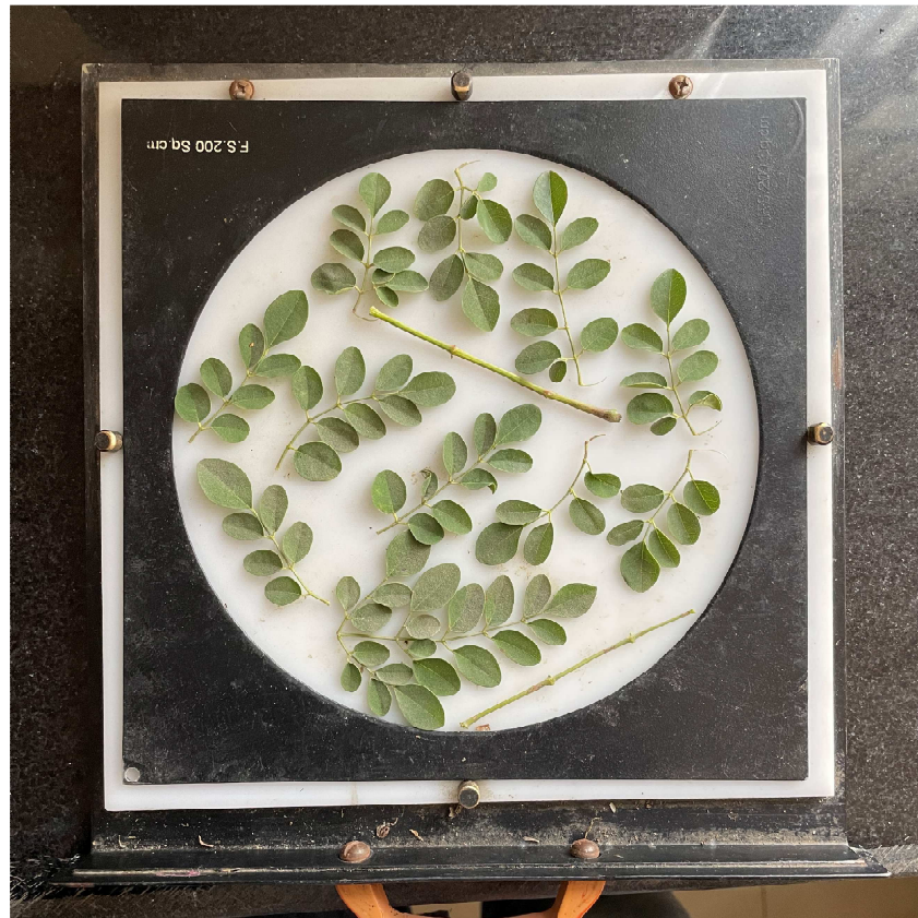
Plate: 5. Measuring leaf area using leaf area meter
