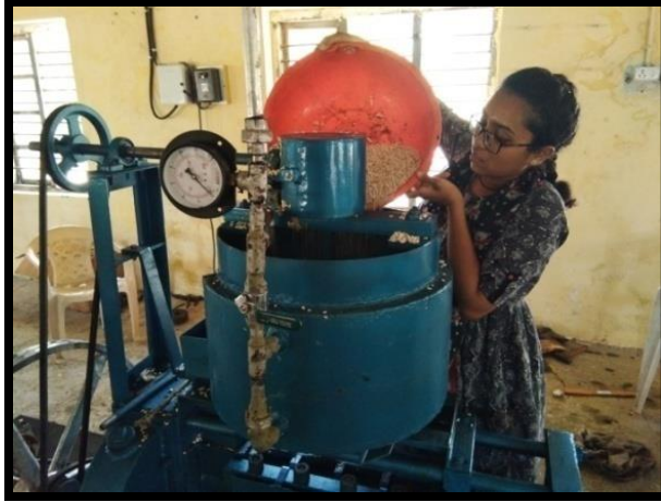
Plate 3.8 Feeding safflower seeds to feed kettle
