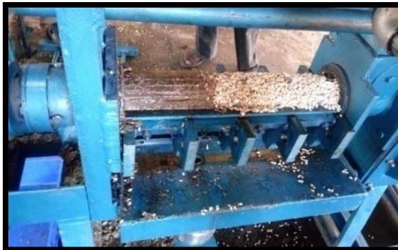
Plate 4.1 Hardened cake at minimum length of reverse worm and low shaft speed
