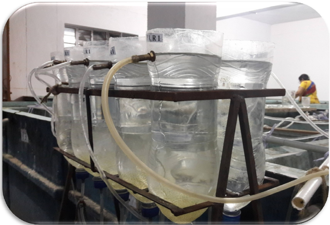
Plate 3.2 Simple hatching device fabricated for egg incubation
