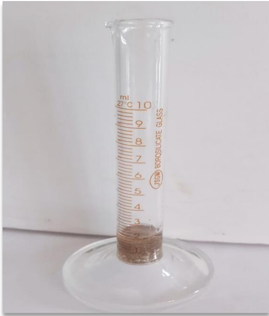
Plate 6. Determination of true density
