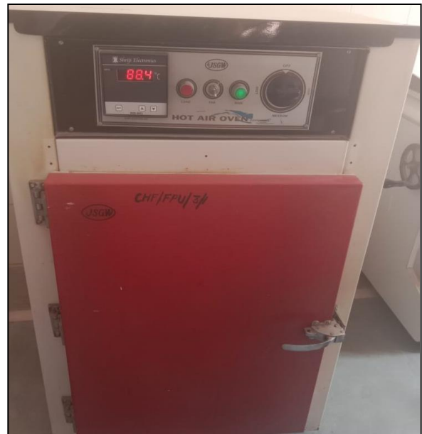
Plate 10. Determination of moisture content
