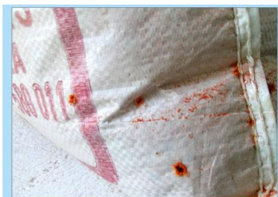
Bore holes of insects in HDPE bag stored at room temperature
