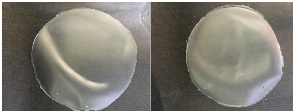
Figure 4.1: Film prepared by corn starch & Glycerol @5 and 2%, respectively
