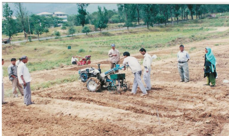
Sowing with power tiller operated zero tillage maize planter
