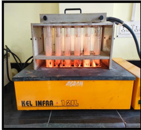
Digestion in block digester
