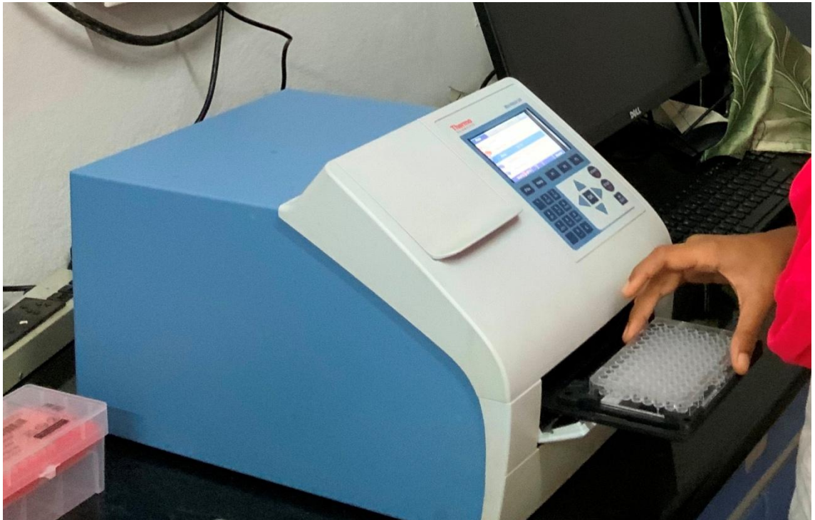
Fig 8. Analysis of serum biochemical parameters using Spectrophotometer
