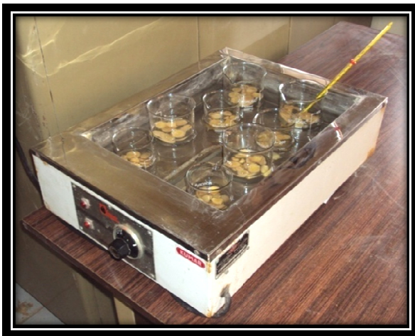
Fig. 3.4: Osmotic dehydration of ginger slices in water bath
