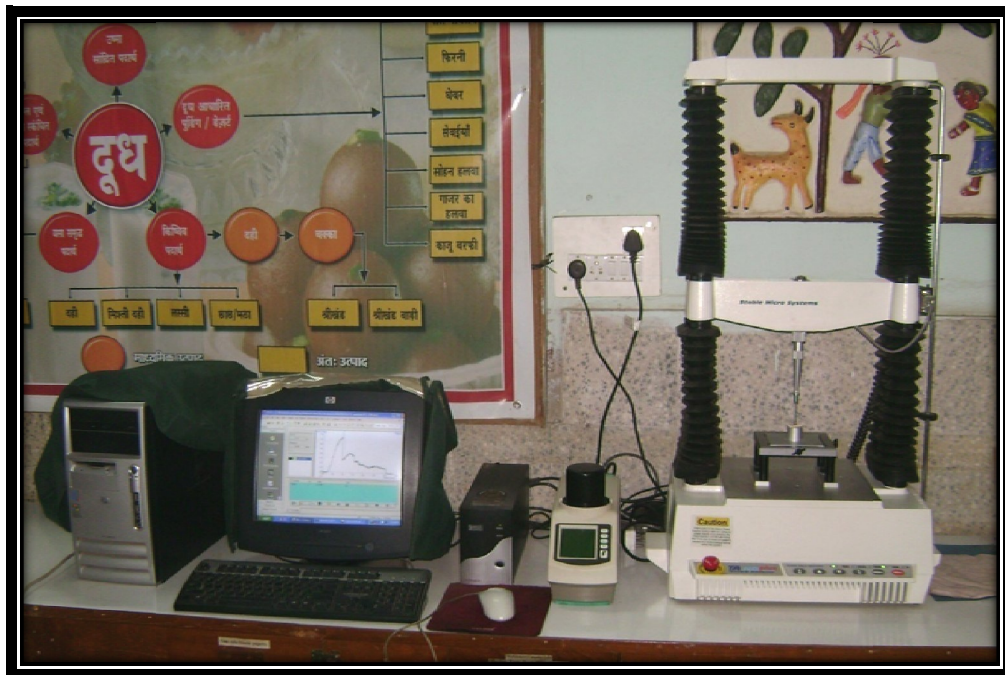
Fig. 3.6: Texture analysis of osmo-air dried ginger slices by Texture Analyser (TA HD Plus)
