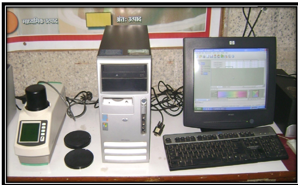
Fig.3.7: Colour observation of osmo-air dried ginger using Hunter lab colorimeter (Colour Flex)
