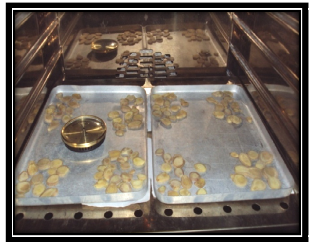
Fig.3.5: Hot-air oven drying of ginger slices
