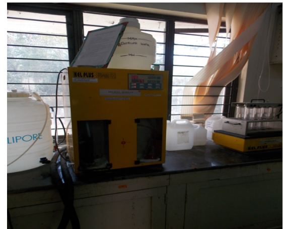
Plate:3.3 (c) sample after digestion Plate:3.3 (d) Distillation of the sample
