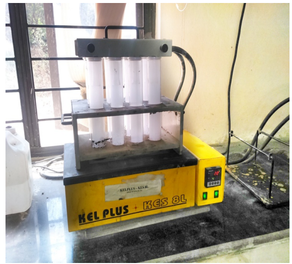
Plate:3.3 (a) Prepared sample for digestion Plate:3.3 (b) Digestion of the sample
