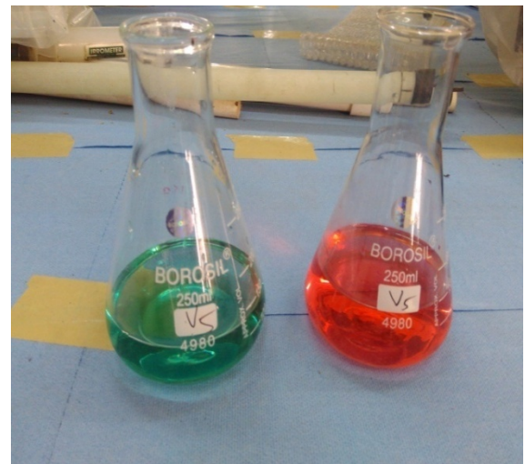
Plate:3.3 (e) Titration with H_2SO_4 Plate:3.3 (f) End point before and after titration
