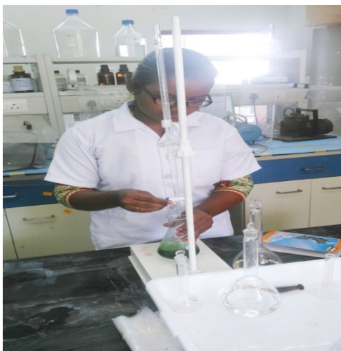
Plate:3.3 (e) Titration with H_2SO_4 Plate:3.3 (f) End point before and after titration
