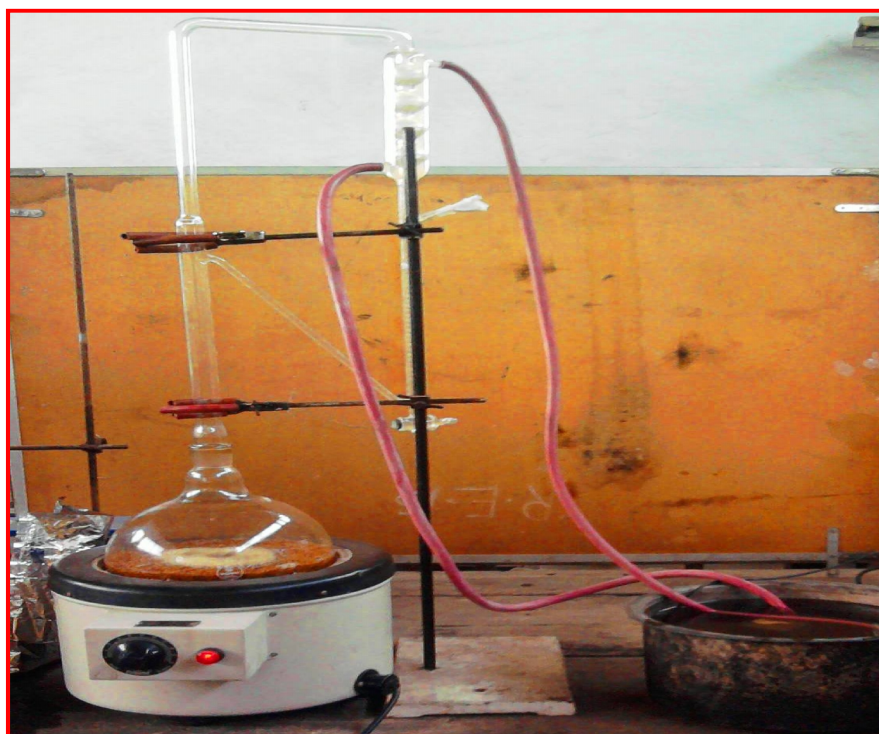
Plate 3.3: Experimental set up of Clevenger apparatus
