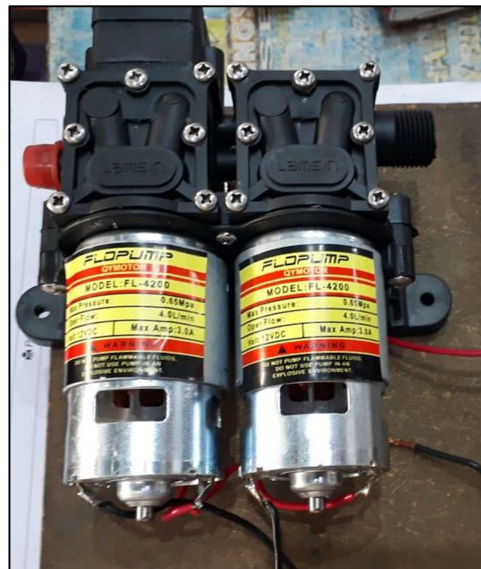
Fig 3.2: Diaphragm pump motor
