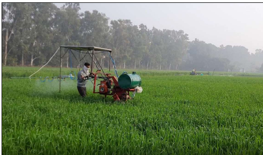
Fig 3.17: Field operation of the solar photovoltaic assisted sprayer mounted on a self propelled carrier
