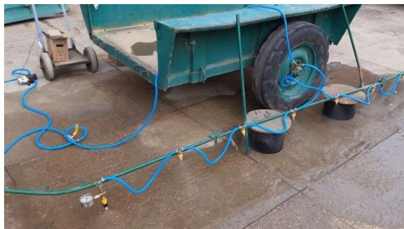
Fig 3.6: Initial testing of the spray boom using battery
