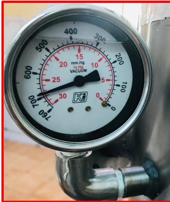
Fig. 3.8 Pressure gauge showing vacuum of 680 mm Hg
