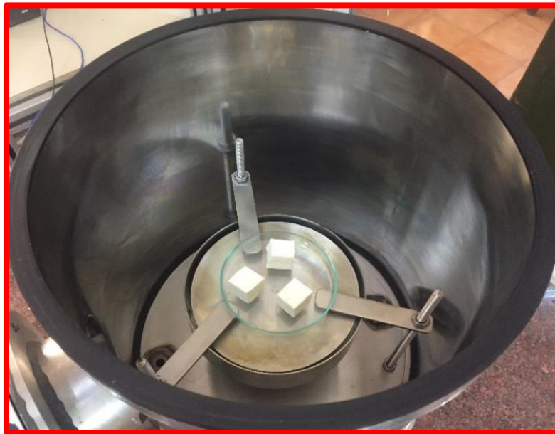
Fig. 3.6 Paneer samples placed on sample holder for treatment
