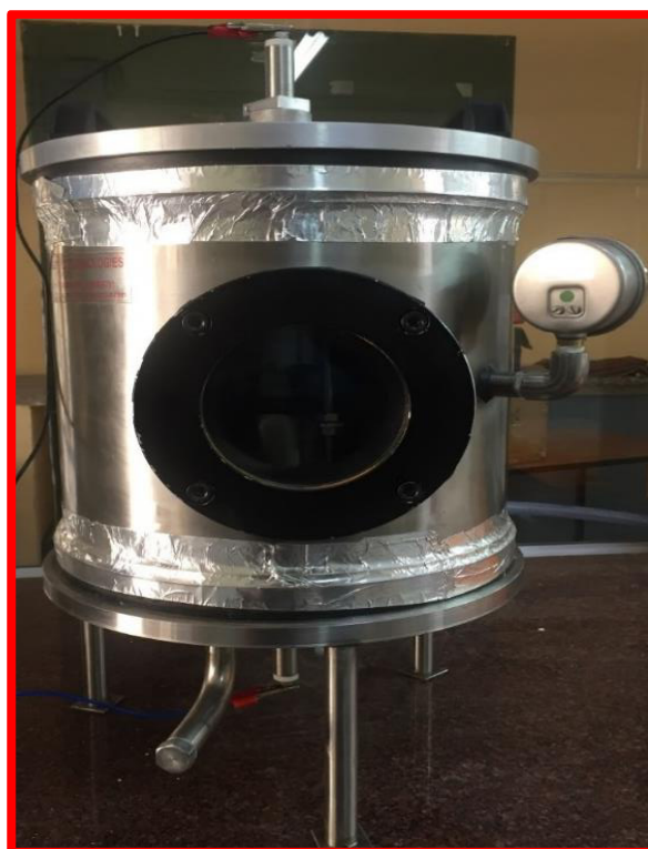
Fig. 3.7 Plasma chamber loaded with paneer cubes for cold plasma treatment
