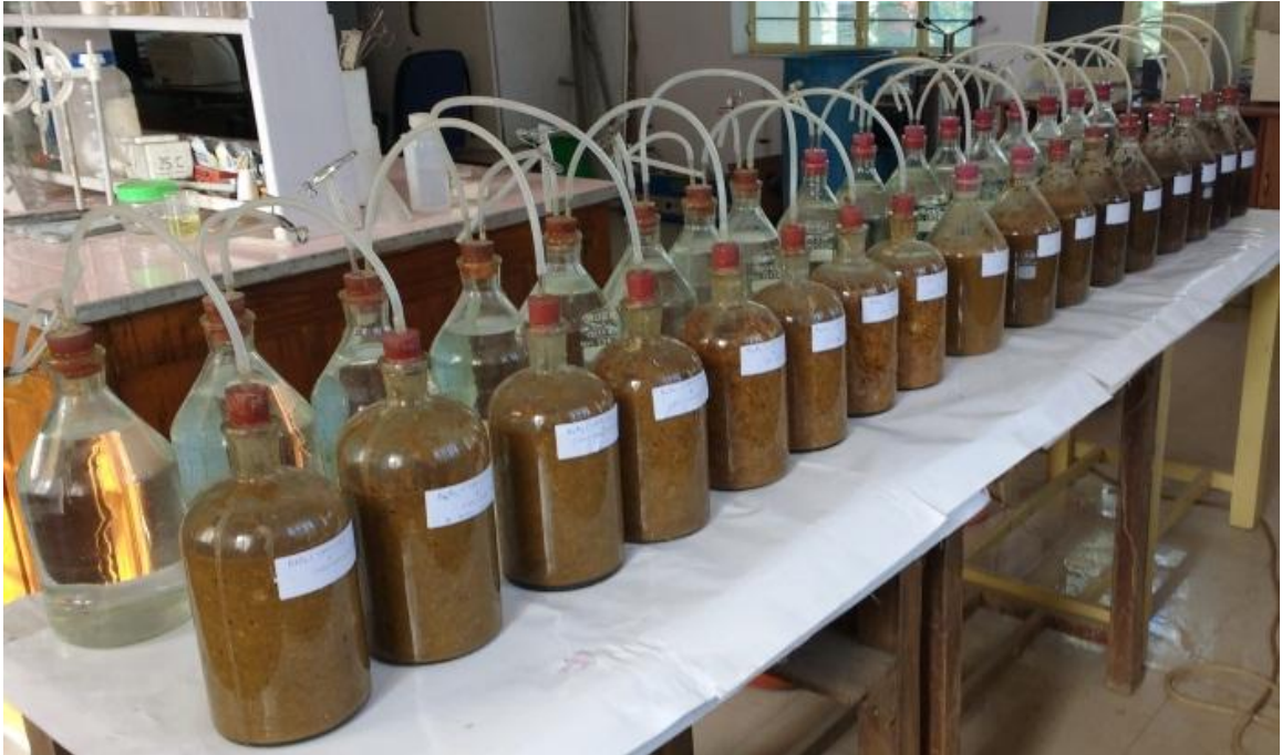
Fig. 3.11a Laboratory set up for biomethanation study of spent mushroom substrate
