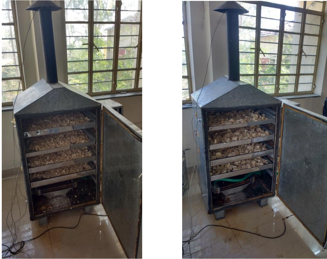
a) Dryer loaded with button mushroom b) Dryer loaded with oyster mushroom
