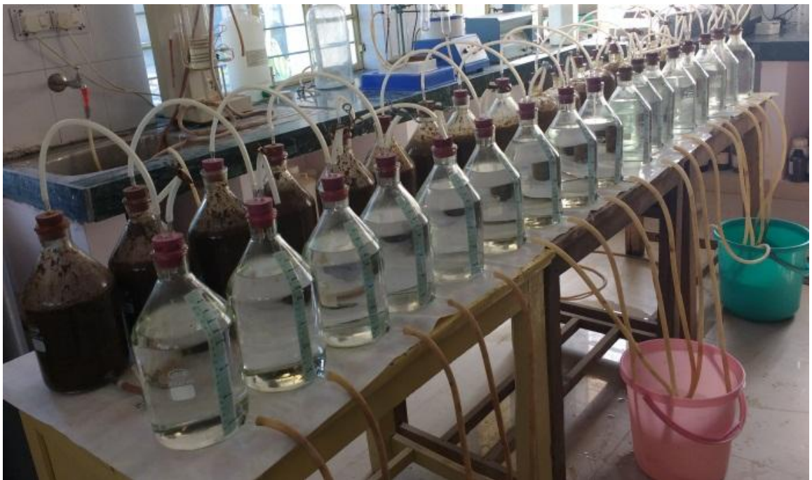
Fig. 3.11b Laboratory set up for biomethanation study of spent mushroom substrate
