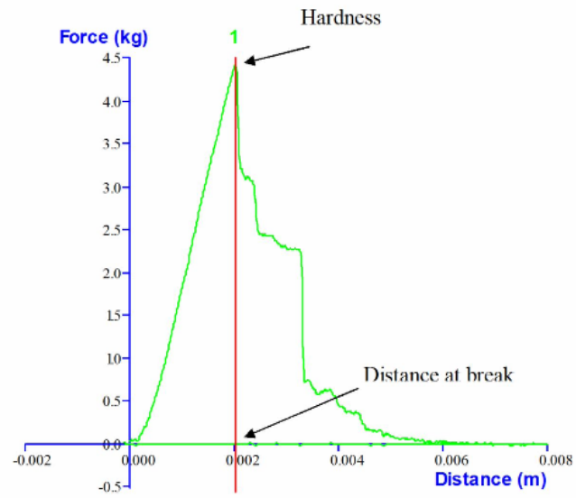
Fig. 3.3 Typical texture profile curve for firmness of biscuits by bending test
