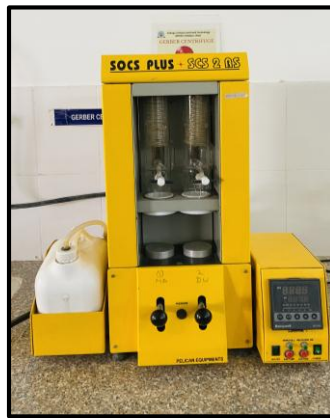
Plate 3.10 Soxhlet apparatus for fat determination
