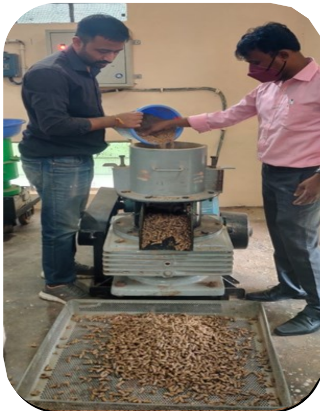
Plate 3 Pelleting of complete feed
