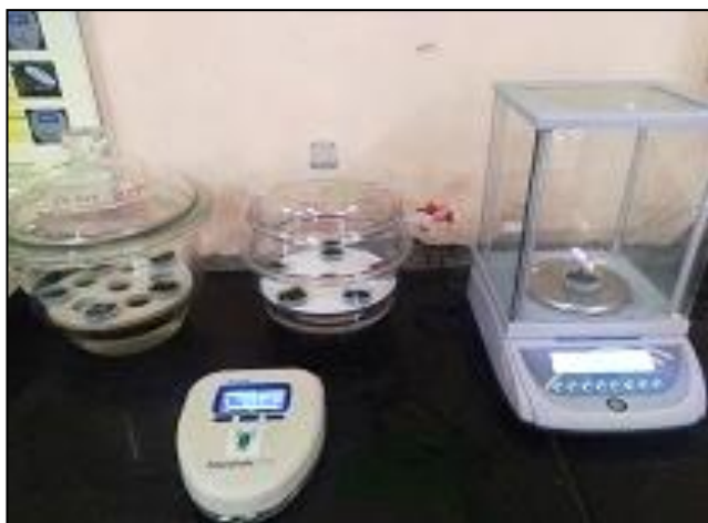
Plate 3.14 Setup for sorption isotherm of final product
