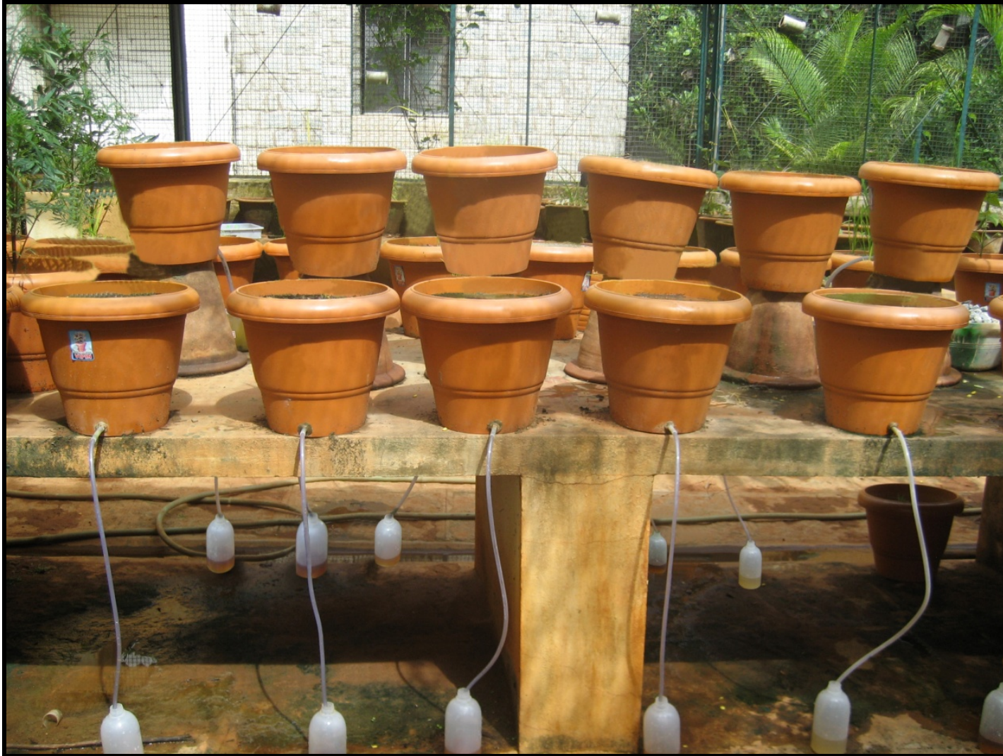
Plate 2 : Experimental set up for reclamation studies and leachate collection
